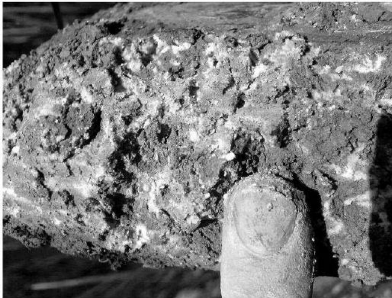
Figure 6.6. Salt crystals (white) marbled in clay loam matrix centered at 60cm depth. Image taken at Mud Slough 3b, 2008.
