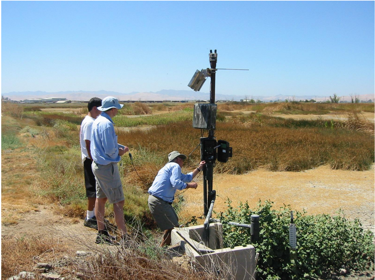
Figure 3.2. MACE USA President Mathew Campbell in the field with Tim Quinlan (sales rep), Ric Ortega (DFG) and Nigel Quinn (photographer) replacing the circuit boards in the Series III instrument boxes to restore output parameters (stage and velocity) and solve the decimal point placement issue .
