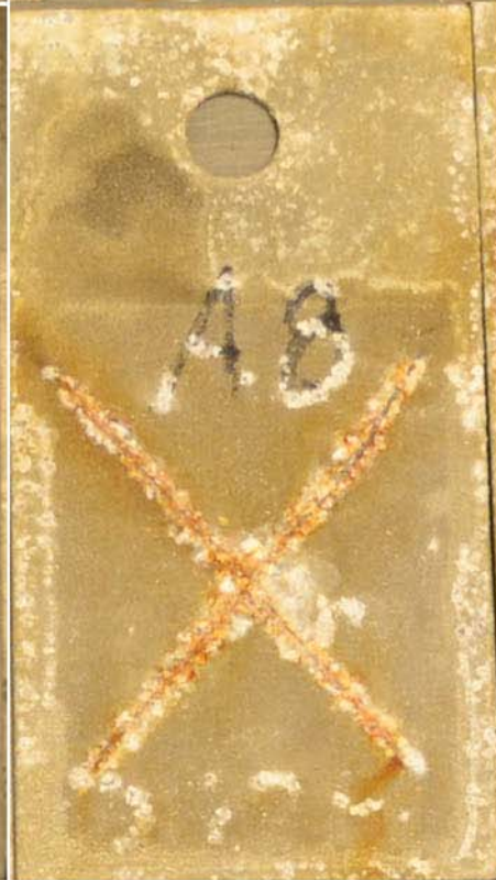
Aluminum – BOR After test (5,040 hours)
