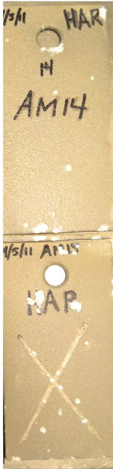
Al/Mg (95/5) – HAR After Test (5040 hrs)
