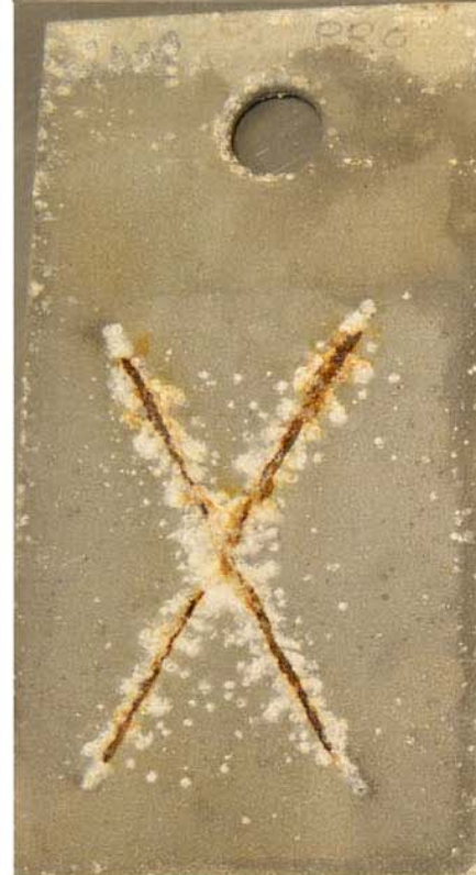
Al/Mg (95/5) – PRO After test (5,040 hours)
