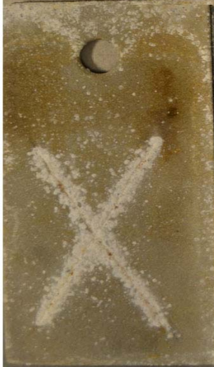
Al/Mg (95/5) – BOR After test (5.040 hours)
