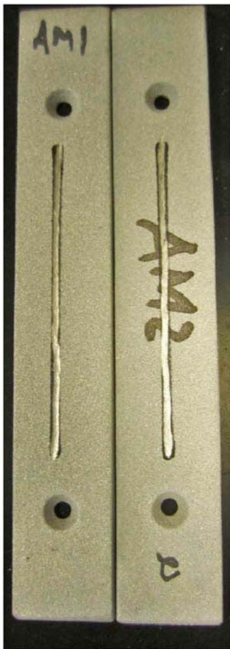
Al/Mg (95/5) - DIFT Before test
