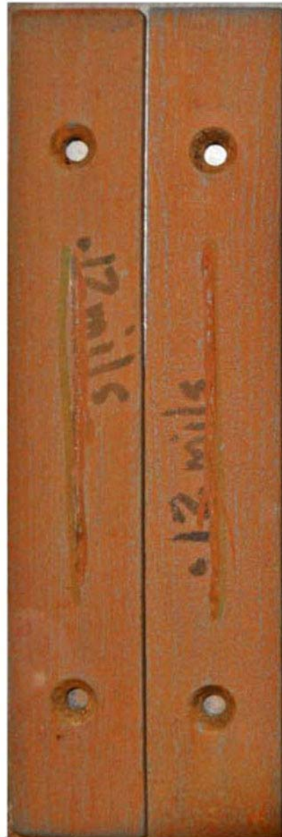
Zinc - DIFT After test (5,040 hours)
