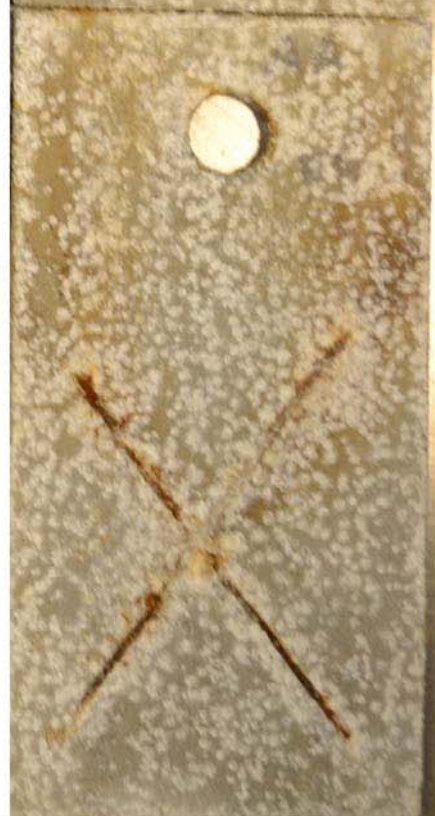
Al/Al 2 O 3 90/10 – PRO After test (5,040 hours)
