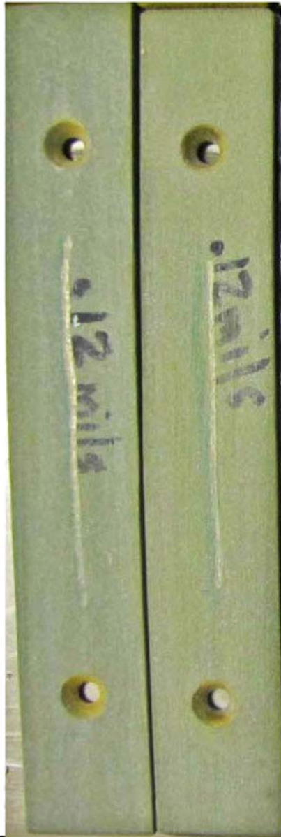
Zinc - DIFT During test (888 hours)
