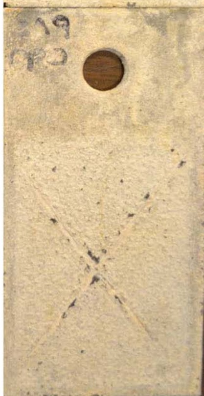
Zn/Al (85/15) – PRO After test (5,040 hours)
