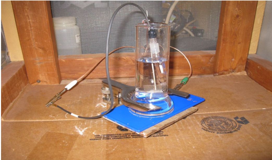
Figure 1.—Experimental setup for EIS.
