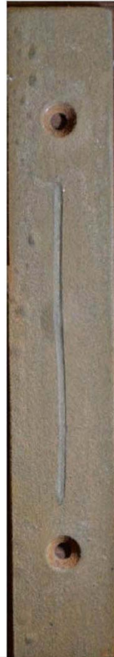
Zn/Al (85/15) - DIFT After test (5,040 hours)
