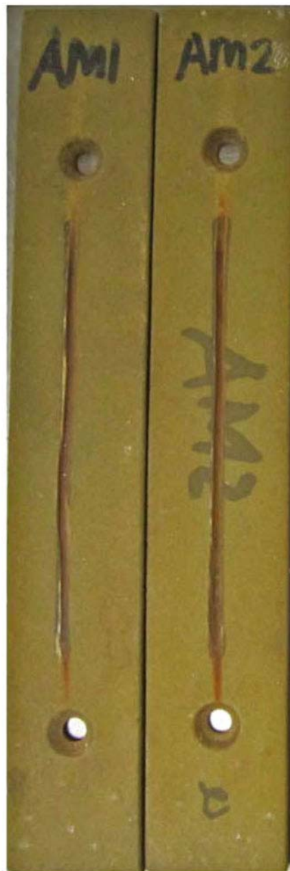
Al/Mg (95/5) - DIFT After test (5,040 hours)
