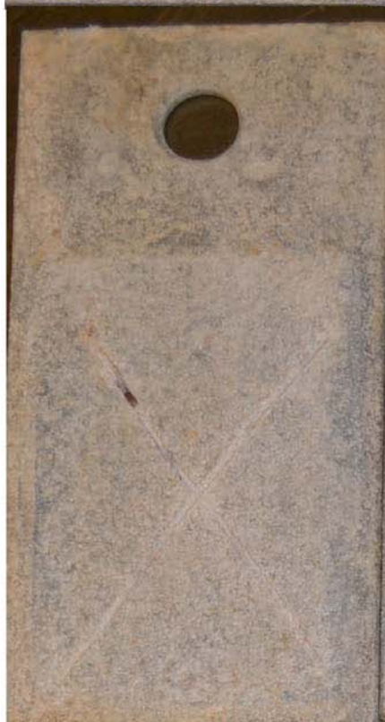
Zinc – PRO After test (5,040 hours)
