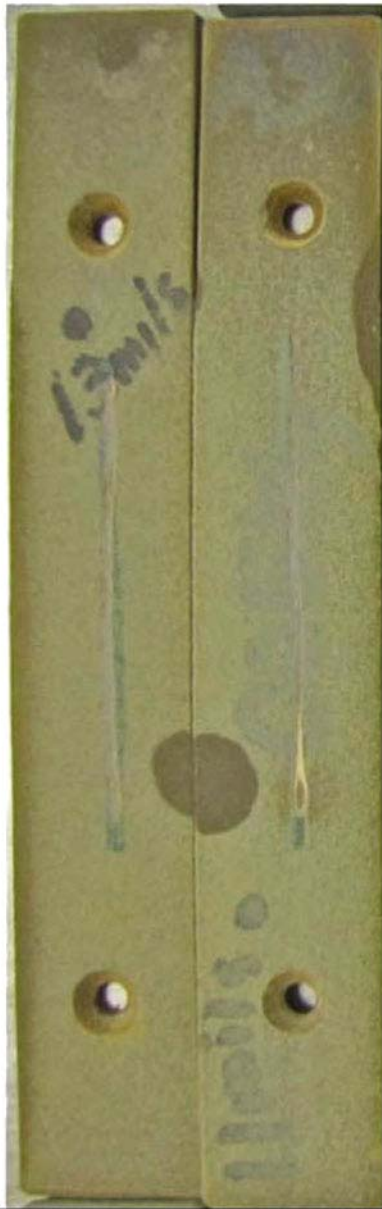
Aluminum - DIFT During test (888 hours)
