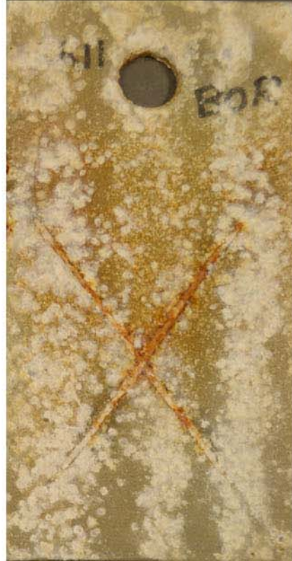
Al/Al 2 O 3 (90/10) – BOR After test (5,040 hours)
