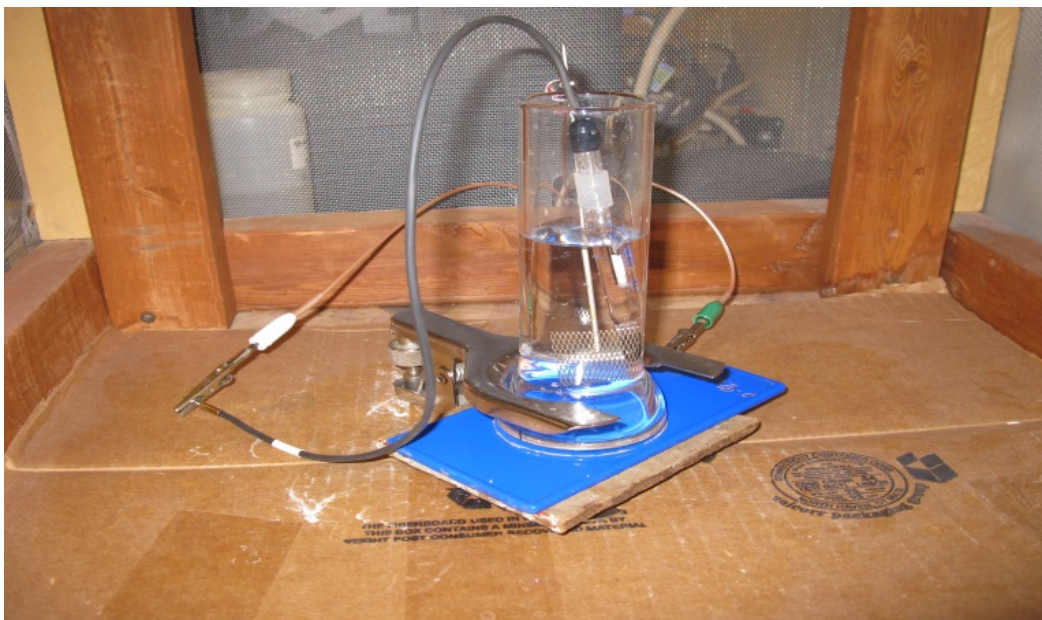
Figure 1.—Experimental setup for EIS.
