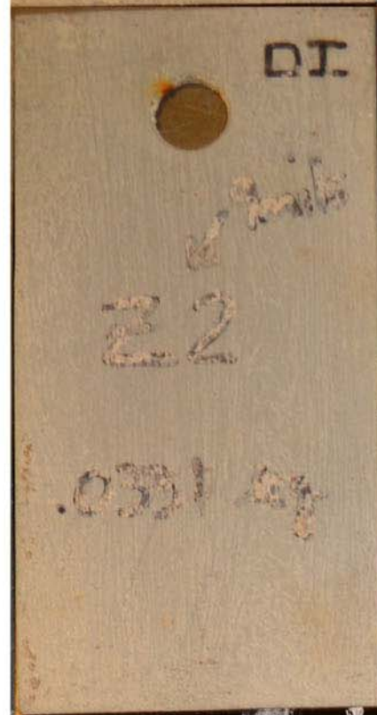
Zinc – DI After test (5,040 hours)
