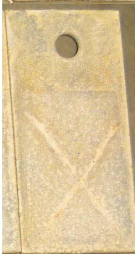
Zinc – BOR After test (5,040 hours)
