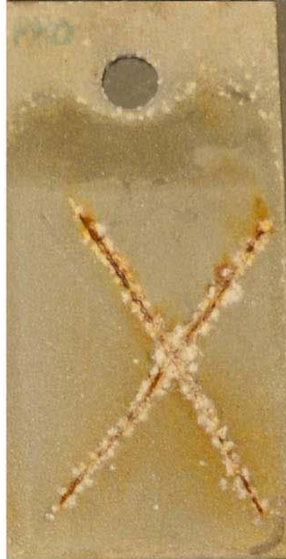
Aluminum – PRO After test (5,040 hours)
