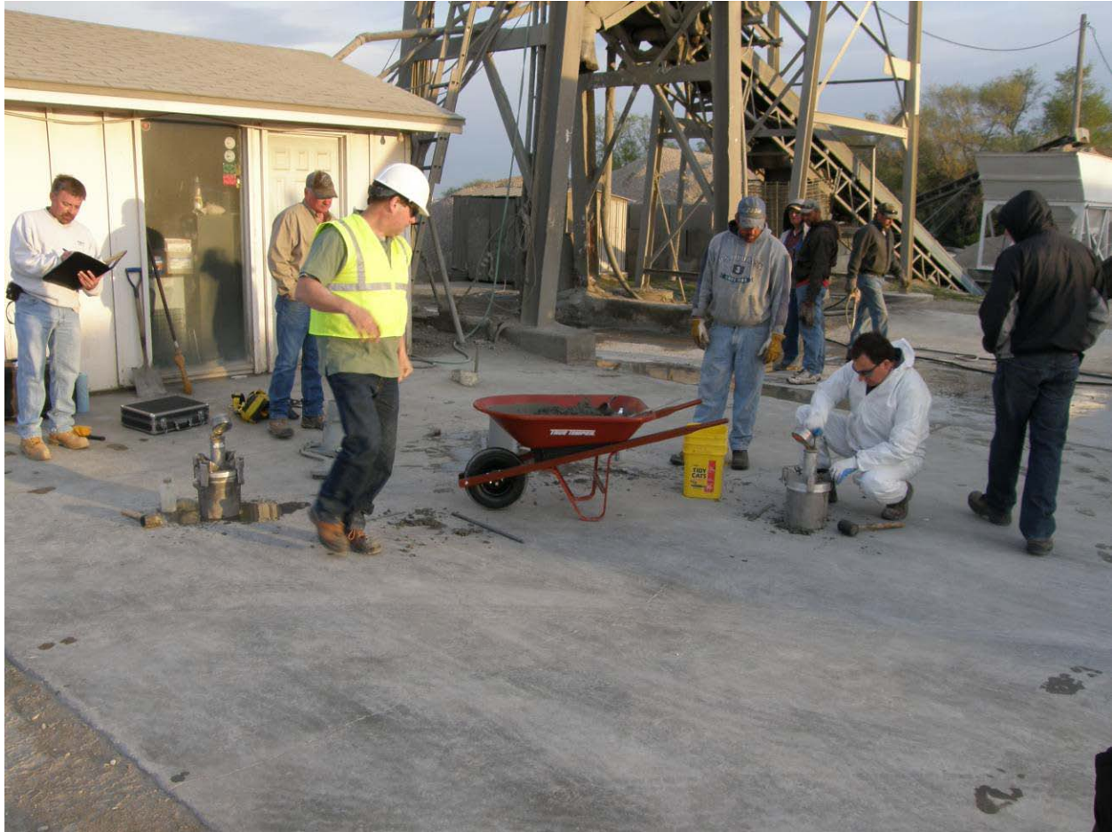
Figure 15. – Measuring fresh properties of the concrete after addition of the Premier Magnesia additive.
