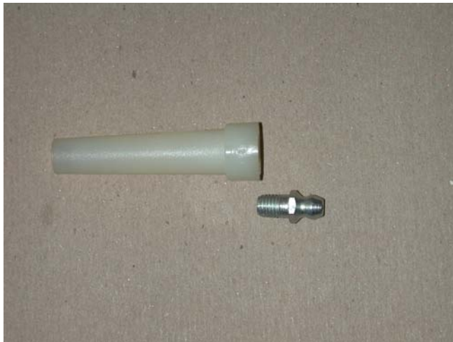
Figure 3. - Example of a bang-in packer with the zirc fitting removed.
