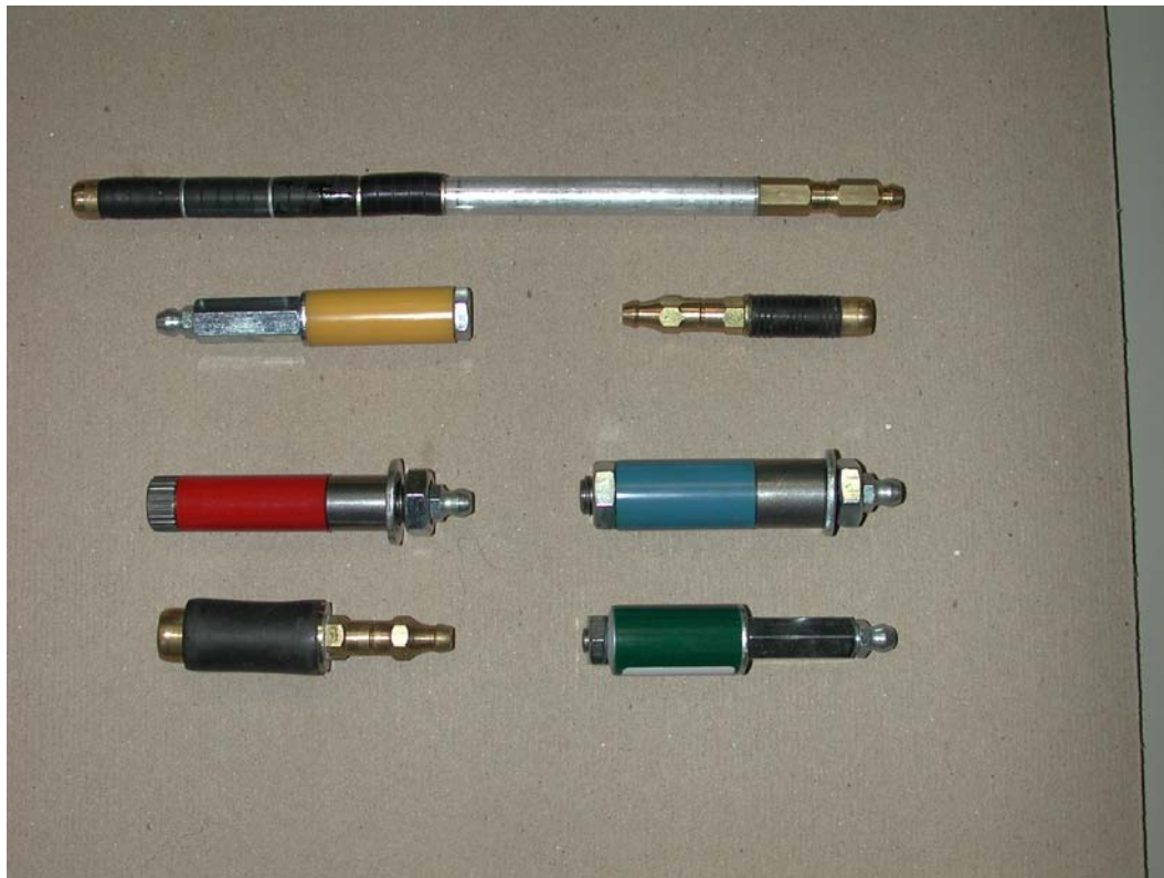
Figure 6. - Examples of mechanical packers. Typically, a nut near the top of the packer is tightened, compressing and expanding the rubber sleeve(s), locking the packer into the hole. Grout can be injected through the zirc fitting.
