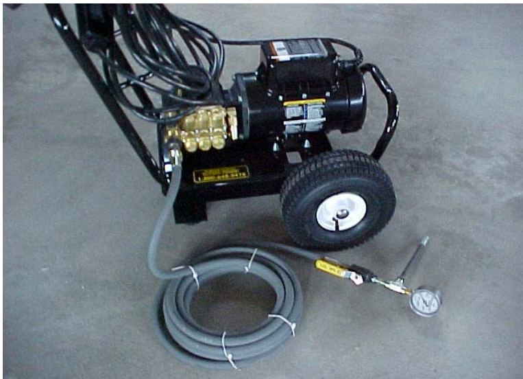
Figure 11. - Pressure washer used to water test cracks.
