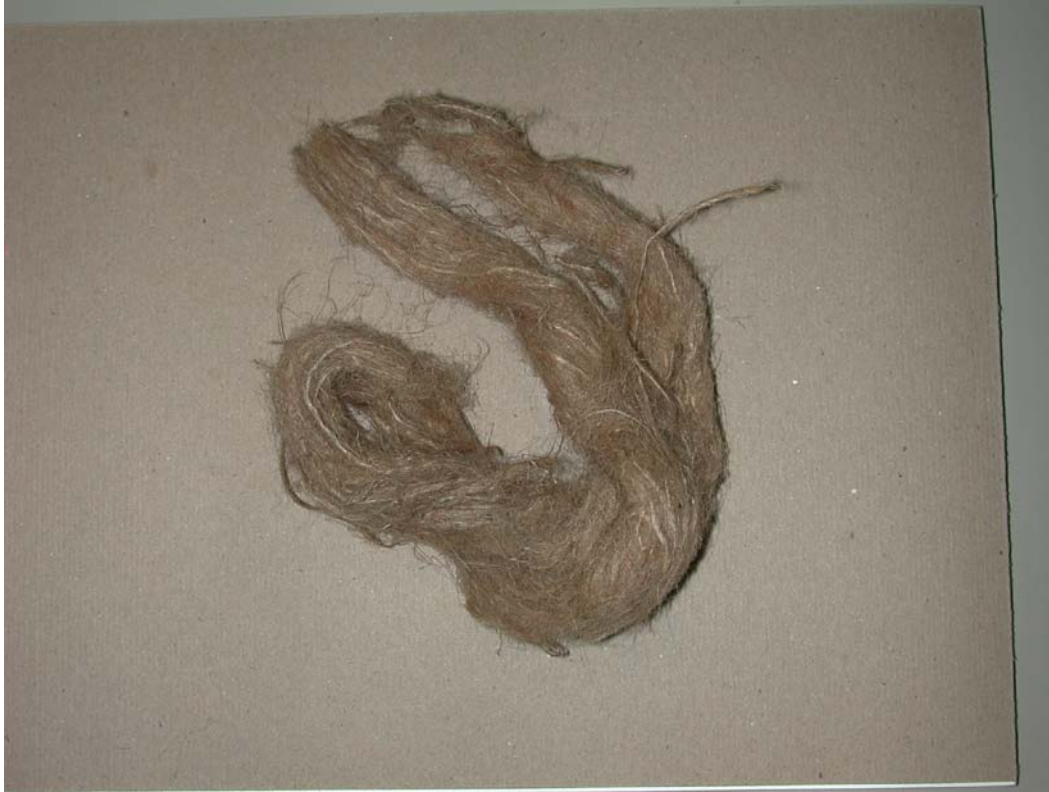
Figure 13. – Jute used to seal crack faces. The jute can be soaked with resin, or resin and water depending on the system, then pounded into the crack opening.
