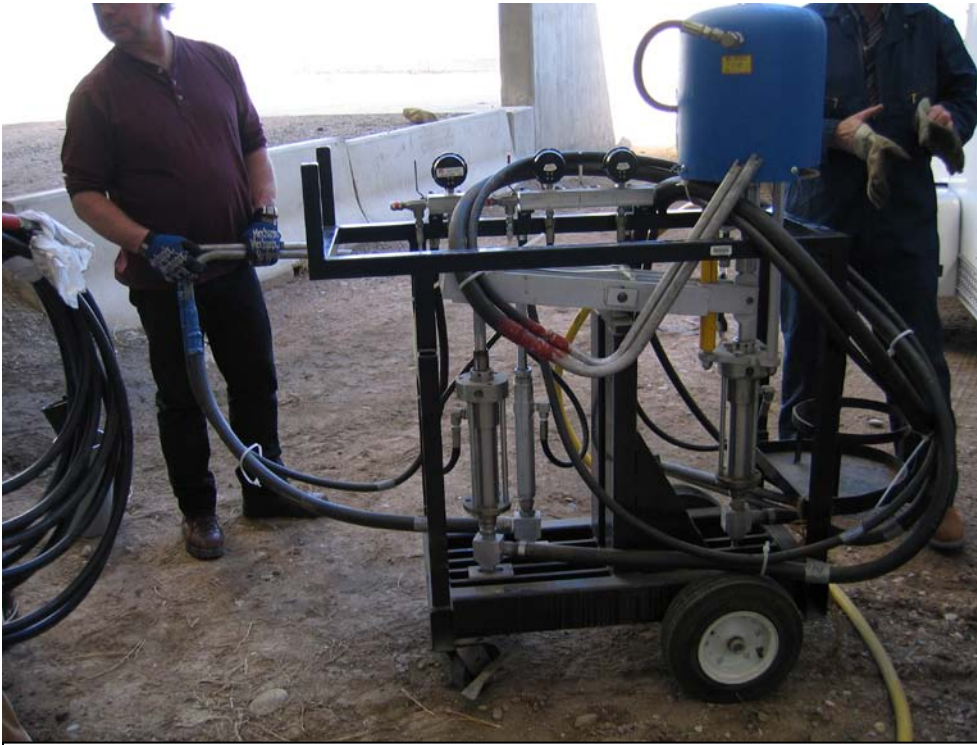
Figure 4. - Multi component, variable ratio, rocker pump.
