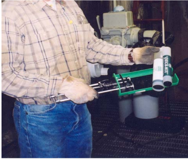
Figure 2. - Hand held, caulk gun injection system.
