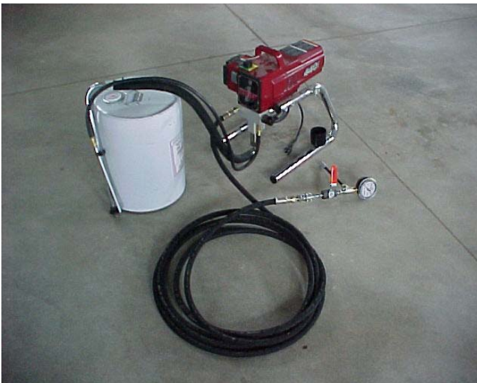
Figure 3. - Modified paint sprayer for chemical grout injection.
