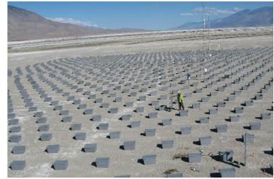
Engineered solid roughness elements test at Owens Lake Source: NASEM 2020, Effectiveness and Impacts of Dust Control Measures for Owens Lake; Photo in report from Holder, 2019d
