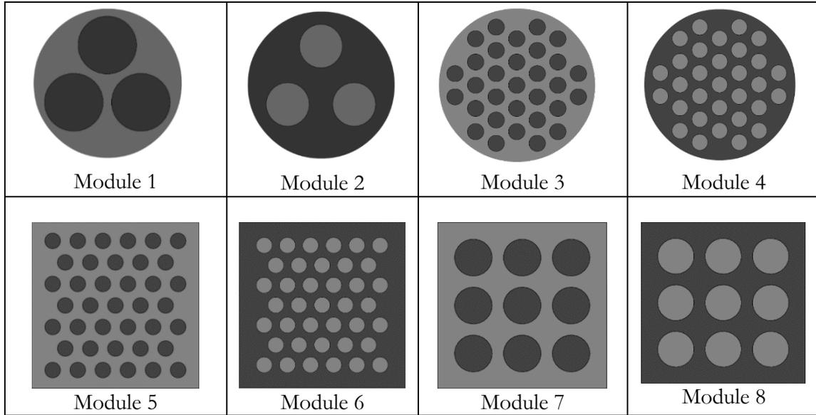
Figure 3. Different containment designs of the TES module. The volume of ROC salt is equal in all cases. Module 8 corresponds to the minimum overall TES cost (baseline) – Dark color: ROC Salt, light color: heat transfer fluid
