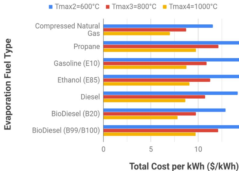
Figure 5. Sensitivity of normalized cost of ROC-based TES system with respect to evaporation fuel type
