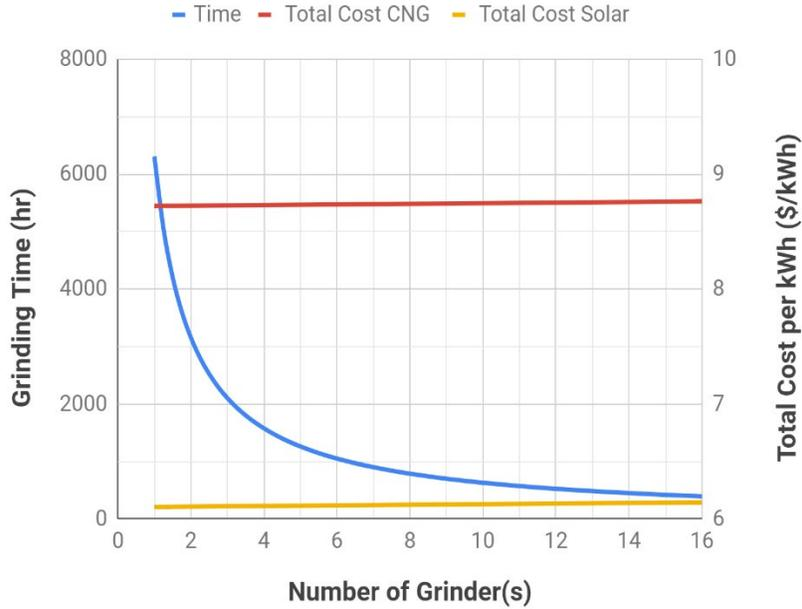
Figure 7. Effect of the number of commercial grinders on the processing time and the normalized cost of TES using CNG and Solar ponds. Baseline case assumes 3 grinders
