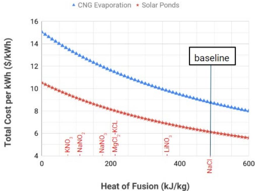
Figure 9. The effect of ROC salt heat of fusion on the normalized TES cost
