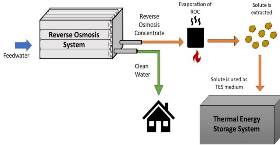
Figure 1. Development of an ROC-based thermal energy storage system
