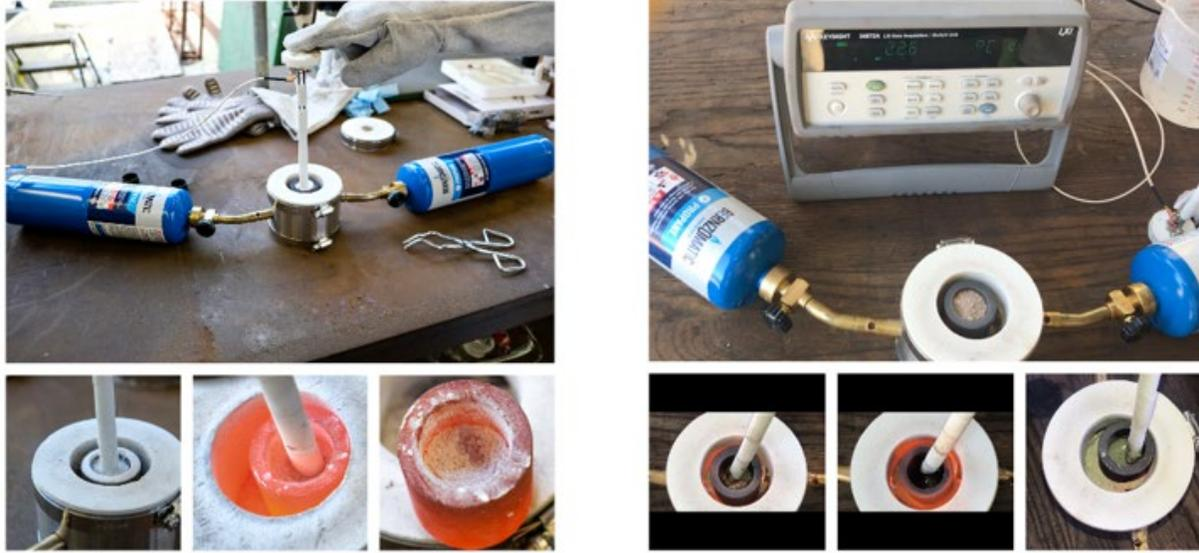
Figure 2. verification of solid to liquid phase change on ROC salt content. No phase change observed in the sample from CDA (left). Solid to liquid phase change observed in the sample from EMWD between 350-400 °C (right)
