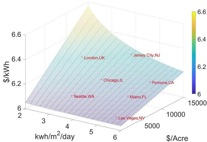
Figure 6. Normalized TES cost using evaporation ponds in different locations. Cost is plotted with respect to local cost of land  $C_l$  and solar irradiance,  $I$
