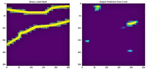
Example automatic crack mapping data set: input (left), label mask (center), and output prediction (right).
