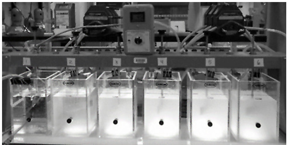
Jar test set up for reactors in series.
