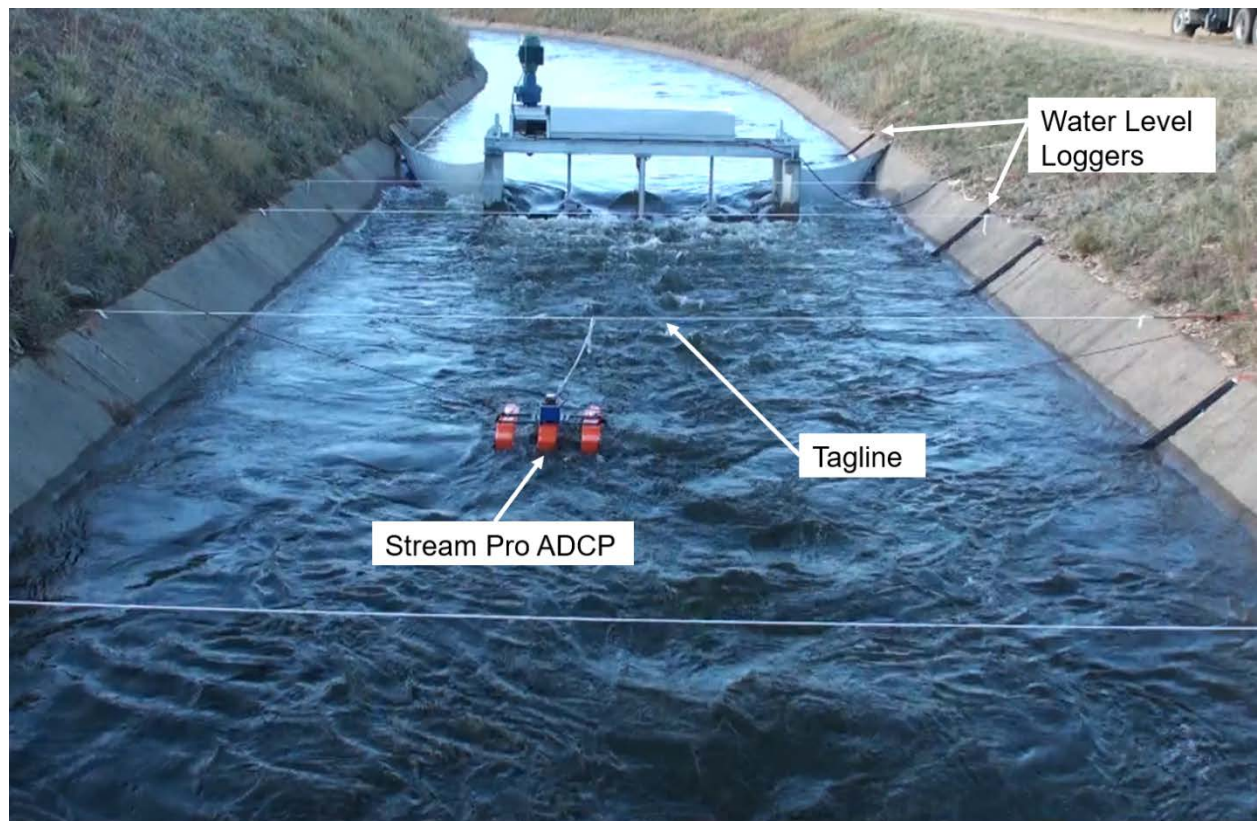
Figure 7 StreamPro ADCP mounted on a tagline for traversing velocity measurements downstream of HK #5.
