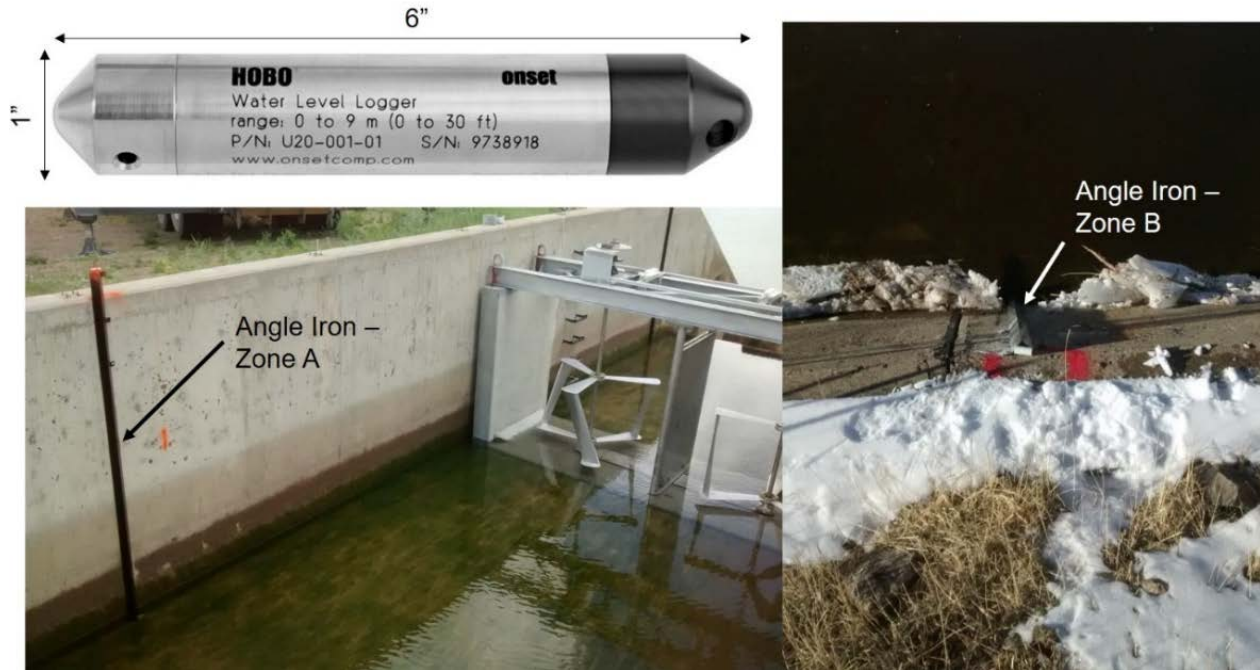
Figure 6 HOBO® water level logger used for water level measurements (top left). Angle iron installations mounted in Zone A (bottom left) and Zone B (right).
