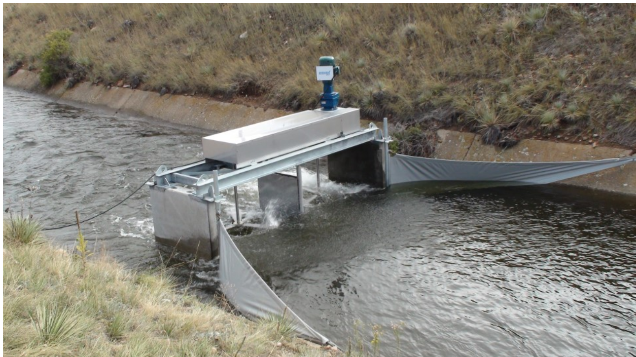
Figure 5 HK unit in operation with temporary upstream transitions made of tarps. Flow is from right to left.
