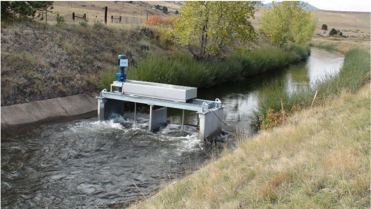
Figure 38 HK #10 with no transitions (Zone B station 2,045 ft at connection with Zone C) operating at 266 ft 3 /s, looking upstream.
