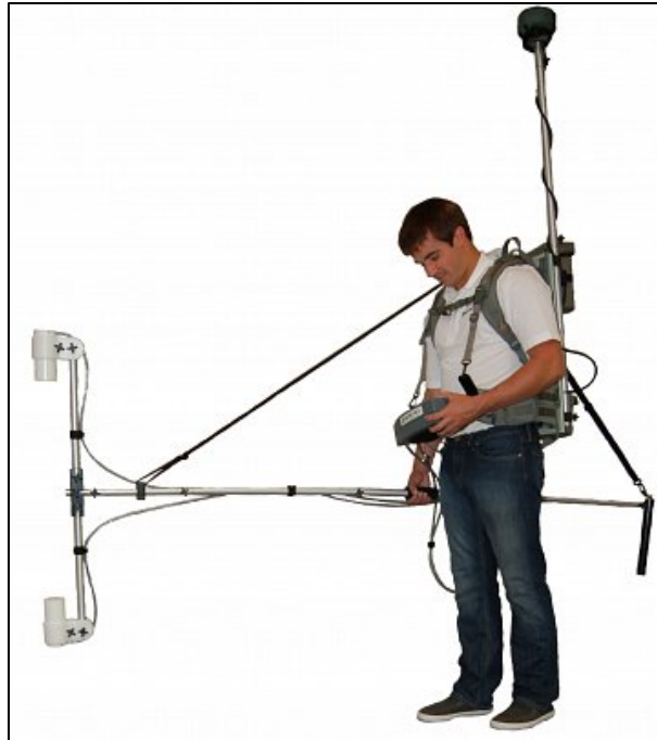
Figure 9. Photo of a Geometrics Inc. G858 magnetometer system configured in a vertical gradiometer fashion, with two cesium-vapor magnetometer sensors vertically aligned one half meter apart, and with DGPS positioning.
