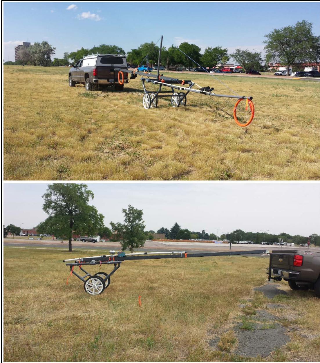
Figure 10. Two photos showing the first iteration of the non-magnetic cart design, being towed behind a truck at the DFC test-site while carrying an EM34 system with 10m coil separation and horizontal dipole orientation (top) and the EM31 FDEM system (bottom).
