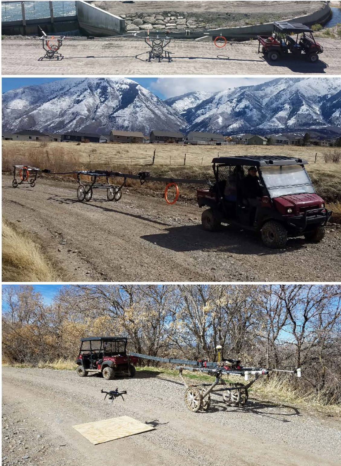
Figure 11. Photos showing the current version of the non-magnetic cart configuration, now utilizing a tethered and gimbaled min-cart for sake of carrying the quite long (~30ft) EM34 system (top two photos). The original main cart is still sufficient for carrying smaller instruments, including the EM38, EM31, and the magnetic gradiometer (bottom photo).
