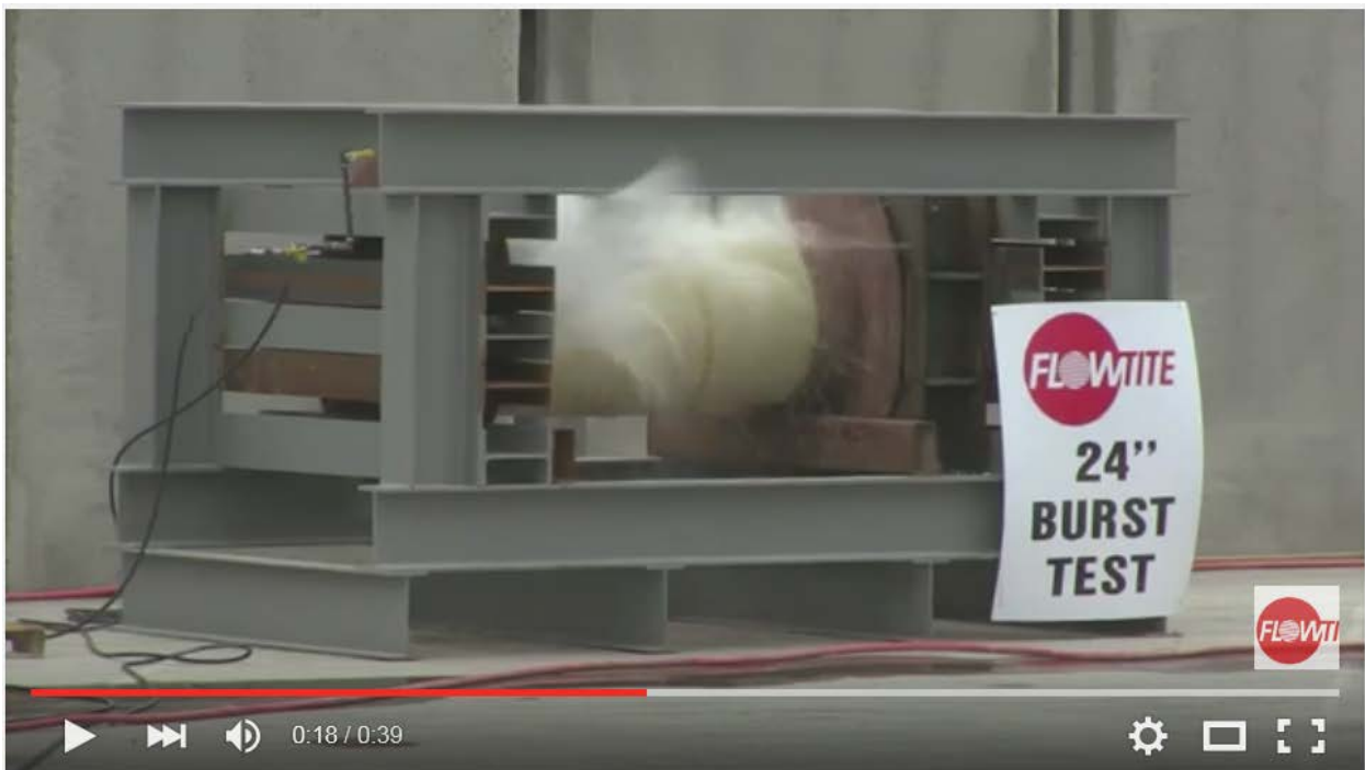
Figure 6 –Laboratory burst test on 24-inch RPM Pipe. Failure initiates at left end cap.
