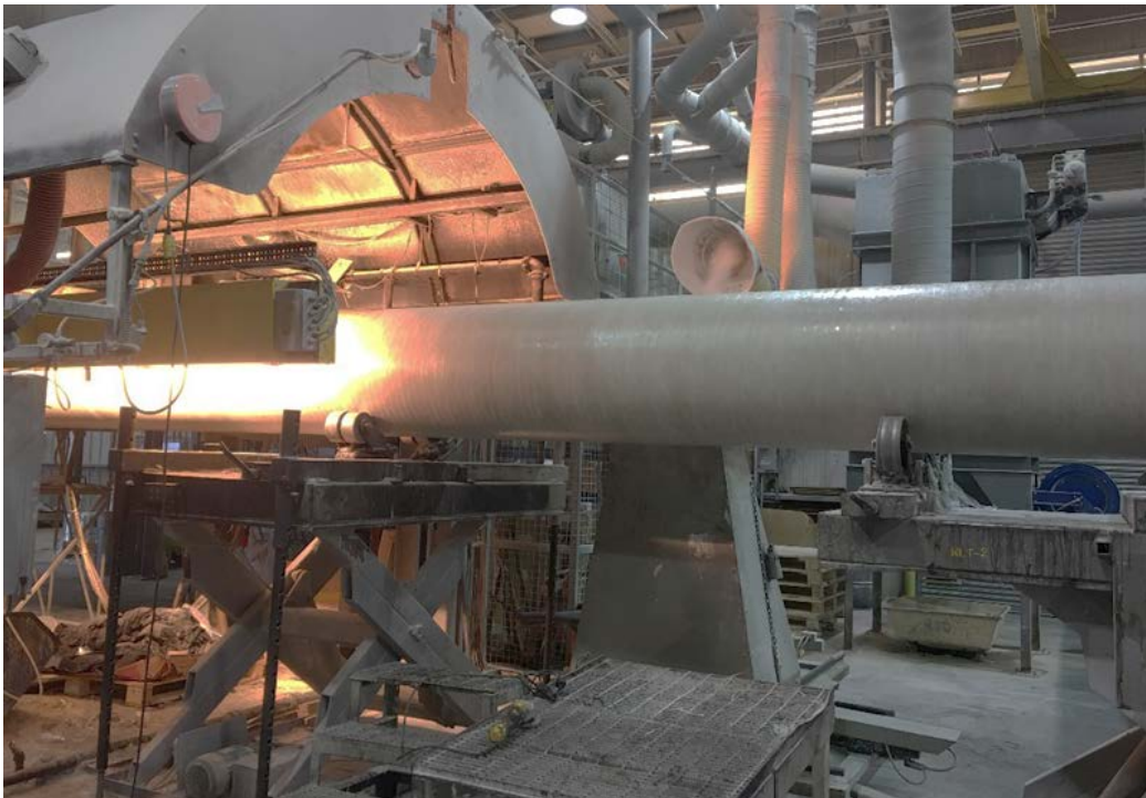
Figure A-6.—Heating system to cure resin
