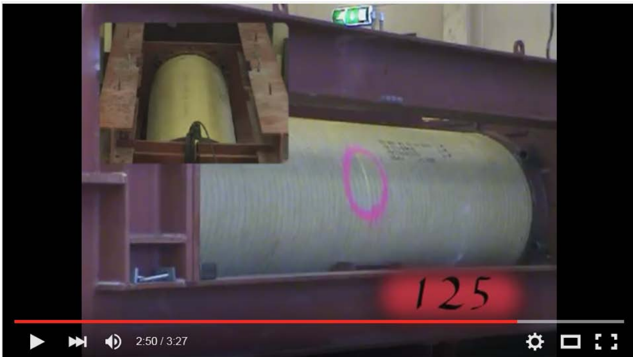
Figure 4 – A split-second prior to failure, a crack appears at the location of the rock impact.
