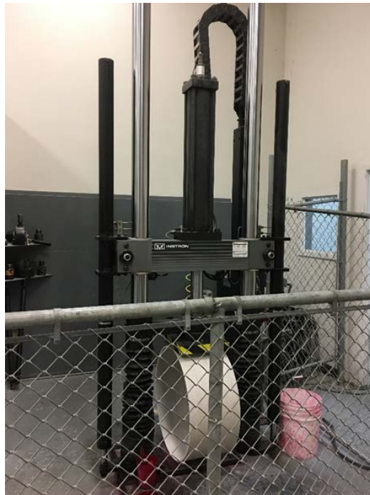
Figure A-13.— Mechanical properties tester (29,000 N load at 5% deflection)
