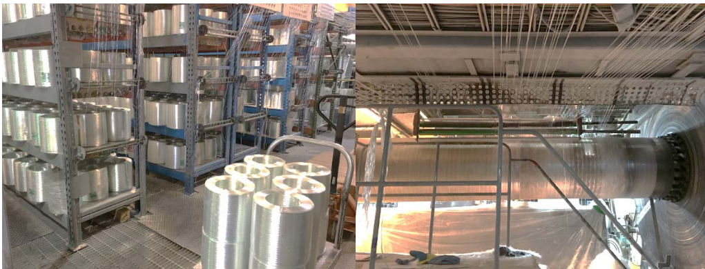
Figure A-4.—Continuous fiberglass thread woven and wrapped over Mylar
