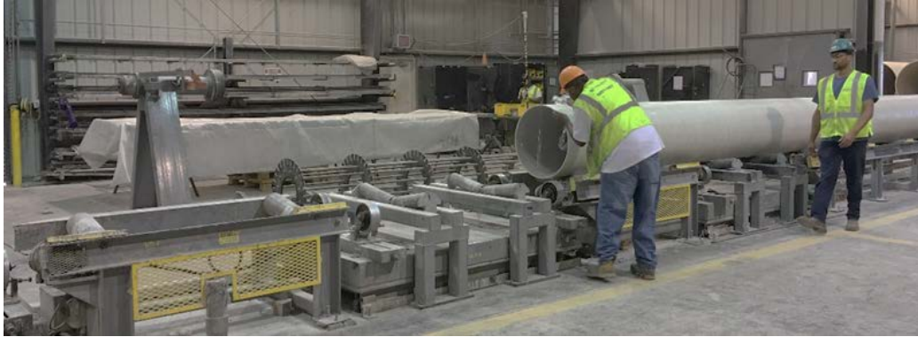
Figure A-9.—Checking the pipe and removing Mylar
