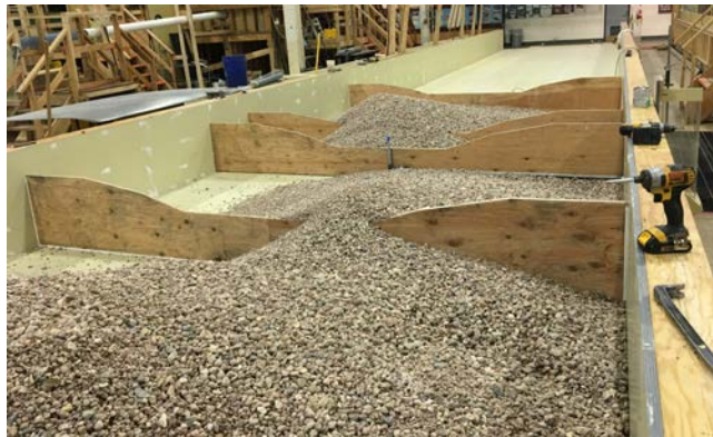
Figure 31. Template system used in model construction to ensure changes in slope remained accurate to prototype
