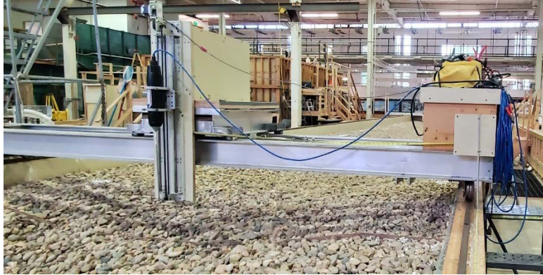
Figure 34. ADV mount in the physical model. The ADV could move horizontally along the length of the model via a traversing system and laterally across the mount by pullies. Additionally, the ADV could move vertically via a stepper motor.
