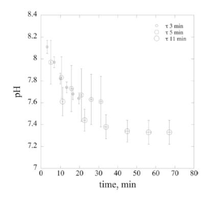
Figure 4. pH vs. reaction time (min). Each data point is a CSTR (nos. 1-6 left to right) for the particular residence time,  $\tau$ . The uncertainties are 1 standard deviation.
