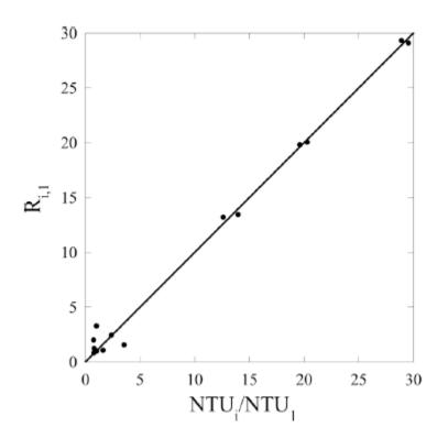
Figure 10. Correlation between predicted ratio of crystal number density and measured turbidity (NTU) using the case of 45 rpm without recirculation as the base case (as defined in equation 13). 45° line drawn to guide the eye.
