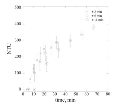
Figure 5. Turbidity (NTU) vs. reaction time (min). Each data point is a CSTR (nos. 1-6 left to right) for the particular residence time,  $\tau$ . The uncertainties are 1 standard deviation.
