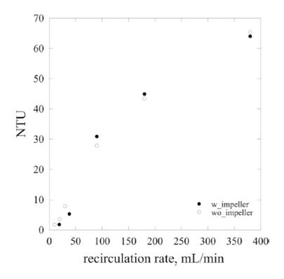
Figure 9. Turbidity in one CSTR using peristaltic-pump-based recirculation mixing with and without additional impeller mixing (@ ~45 rpm) with  $\tau \sim 3$  min.
