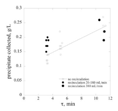
Figure 8. CaCO<sub>3</sub> precipitate collected from 6<sup>th</sup> CSTR vs. residence time with and without recirculation mixing in the 1<sup>st</sup> CSTR. Trendline presented for the impeller mixing-only data.
