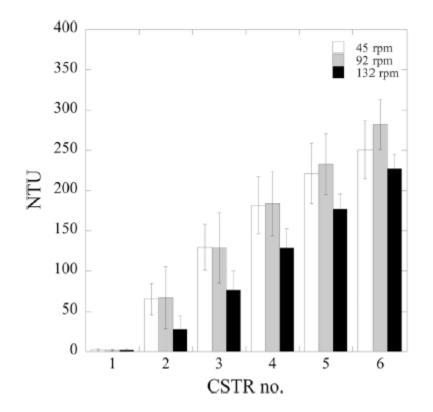
Figure 6. Effect of impeller speeds on turbidity evolution ( $\tau \sim 3$  min).
