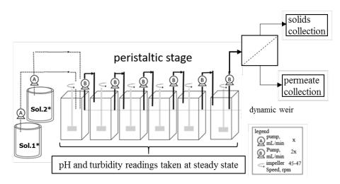
Figure 1. Schematic representation of CSTRs-in-series setup.
