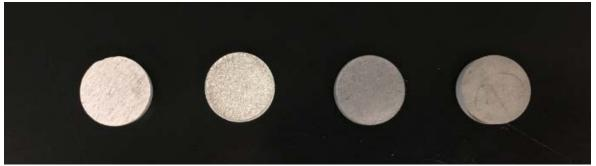
Figure 1: 316L stainless steel specimens. From left: cold rolled steel, as-printed PBF printed steel, heat treated PBF printed steel, and PBF printed steel after sensitization and etching.
