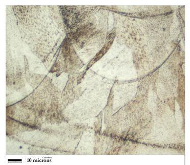
Figure 11: Microstructure of the as-printed specimen at a magnification of 63X.
