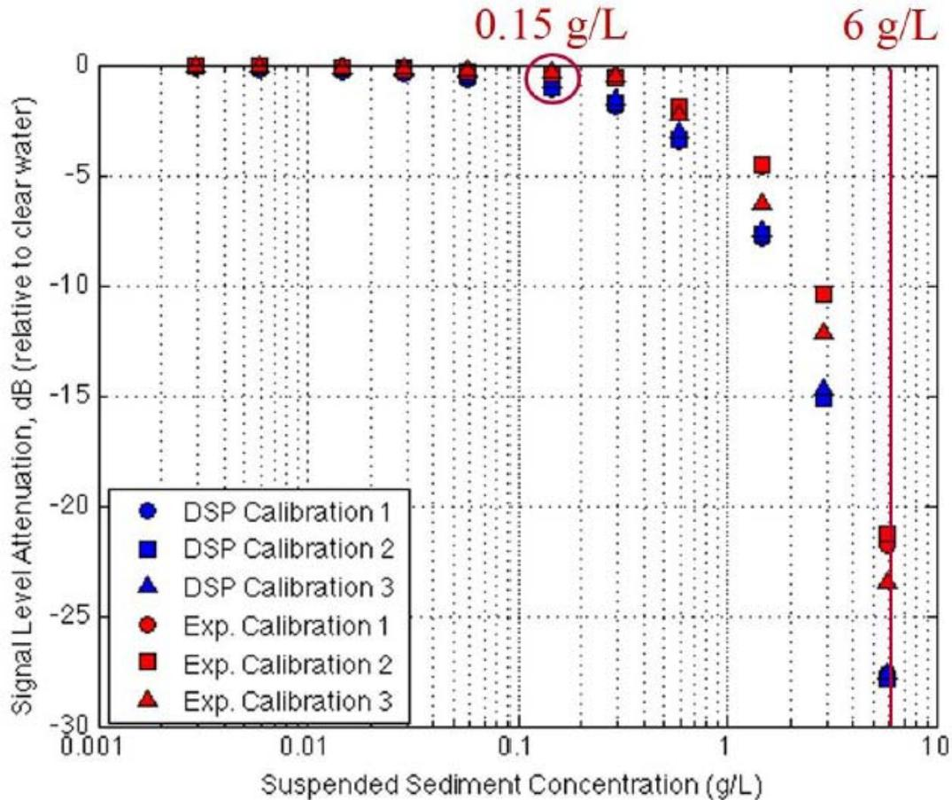
**Figure 24. Laboratory calibration of the NCPA acoustic device, as arranged for the Goodwin Creek deployment. The detectable range for silt sized particle ( $D_{50} = 20 \mu\text{m}$ ) ranged from 0.15 g/L to 6 g/L using the current 18 cm spacing.**
