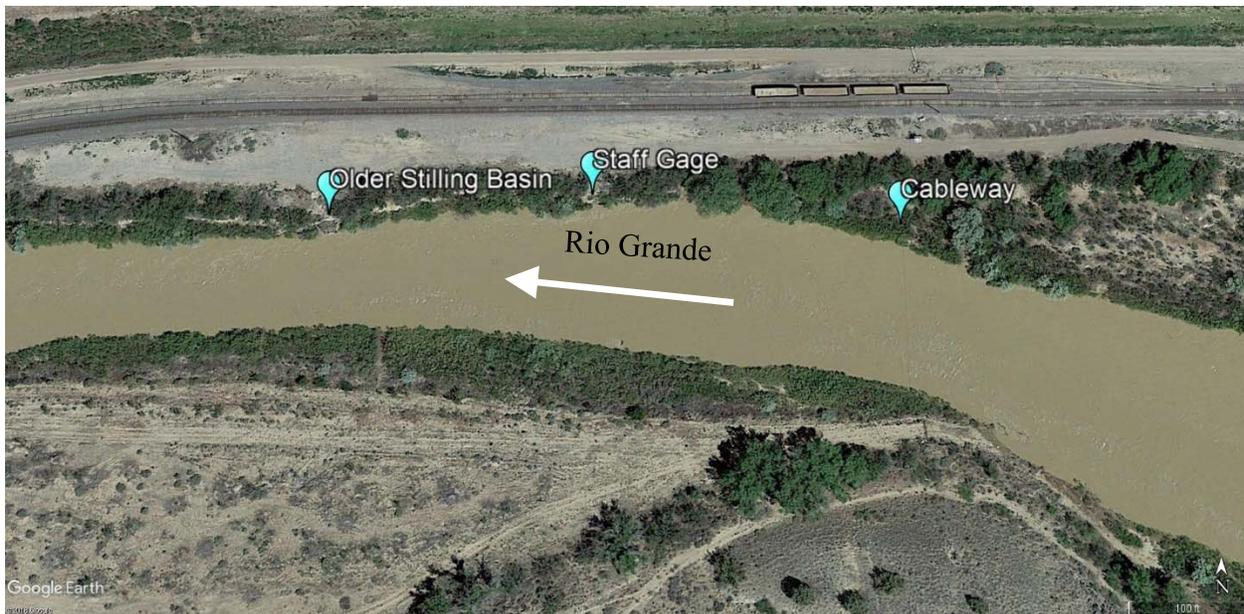
**Figure 1. Potential site locations for locating acoustic sediment instruments at the USGS San Acacia gaging station. Image was created in Google Earth Pro (version 7.3.2.5776) using the 2017 MRG aerial imagery.**
