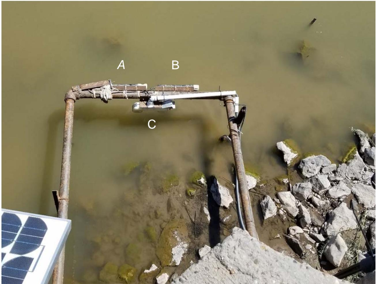
**Figure 13. Active acoustic installations on the Rio Grande at San Acacia: A) 1 MHz and B) 2 MHz AquaDopp acoustical probes and C) NCPA 20 MHz acoustical instrumentation. Photograph taken by W. Carpenter (NCPA) on July 24, 2017.**
