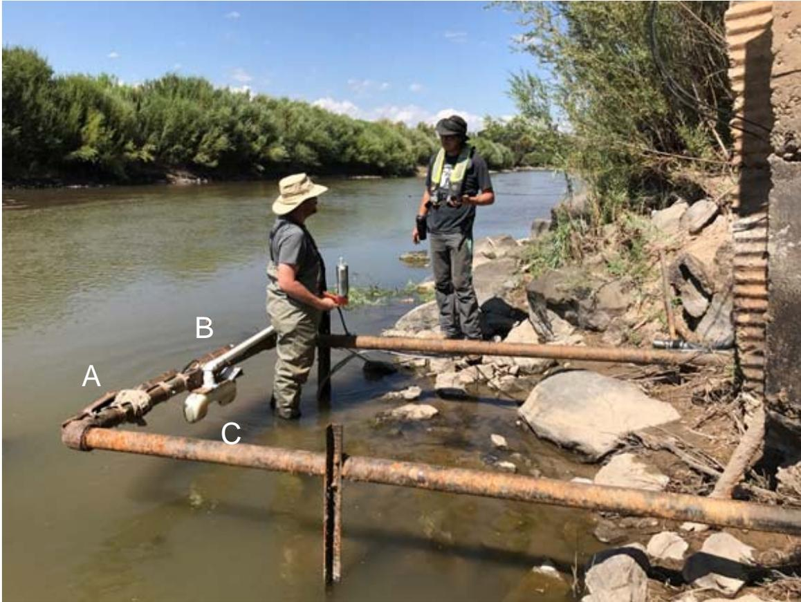
Figure 14. J.D. Heffington (NCPA) and Tyson Hatch (NMWSC), discuss details of the NCPA 20 MHz acoustical instrumentation (C). Previous AquaDopp acoustical probe installations on the Rio Grande at San Acacia are also visible: A) 1 MHz and B) 2 MHz. Photograph taken by J. Brown (NMWSC) on July 24, 2017.
