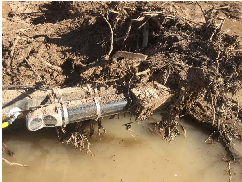
**Figure 18. Debris and sediment left from storm surge on uncontrolled tributaries upstream of the USGS San Acacia gaging station. Shown is the 1 MHz AquaDopp and the upstream angle iron that protected it. Photograph taken by T. Austring, Albuquerque USGS office, on October 13, 2016.**
