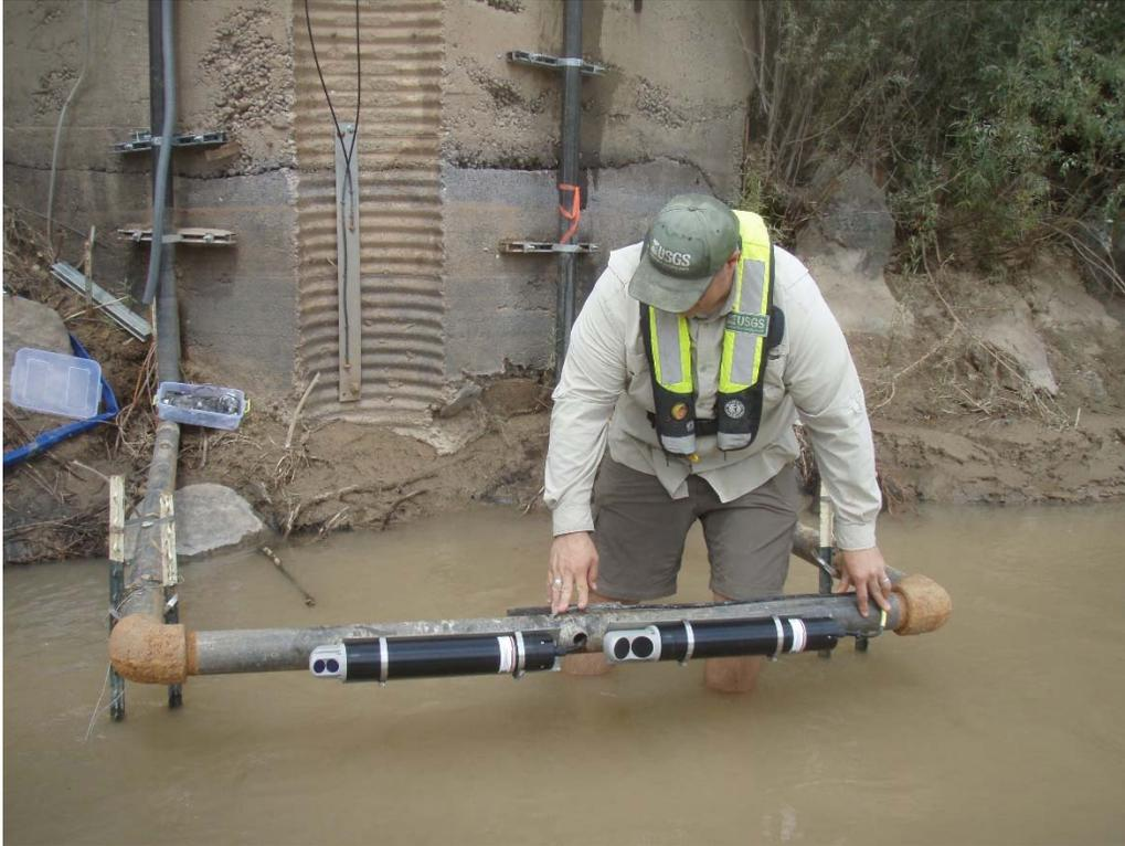
Figure 11. Installation of AquaDopps by NMWSC and GCMRC, looking towards river right bank
