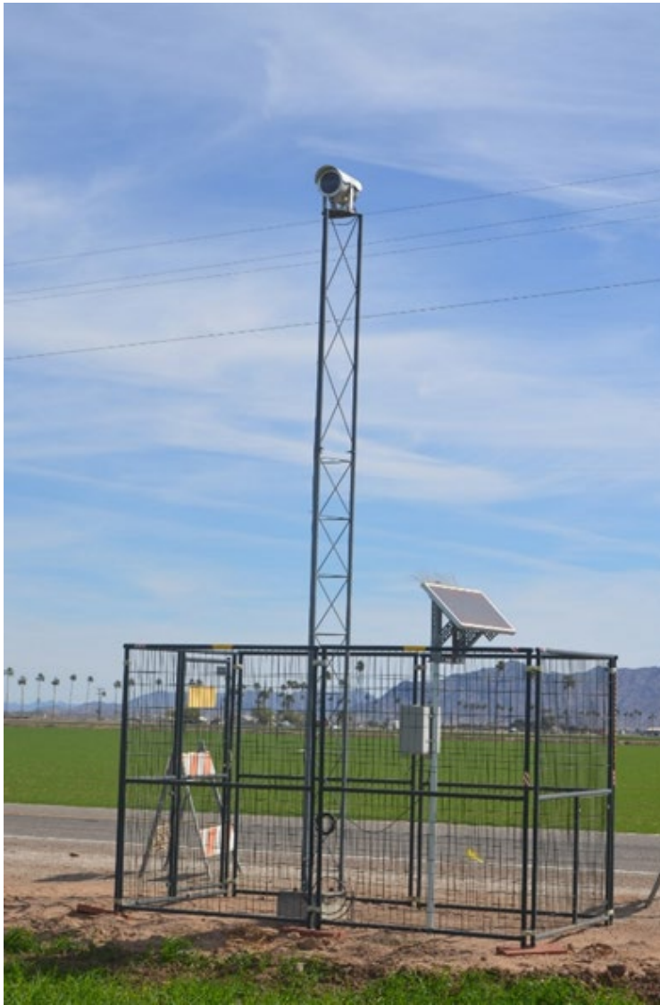
Figure 9. Large Aperture Scintillometer used on durum wheat sites in 2017-2018. Each setup consists of transmitter-receiver pairs, where a collimated beam of near-infrared light is sent across a transect to detect scintillations due to changes in air refractive index. At the sampling wavelength, the scintillations are a representation of sensible heat flux from the soil and crops below the light path. In May 2018, this unit was relocated to a citrus site.
