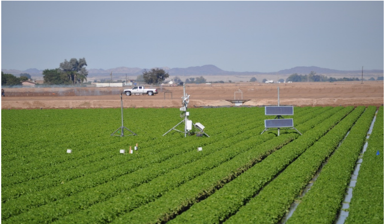
Figure 1. Eddy Covariance (ECV) systems used in field sites for studies.
