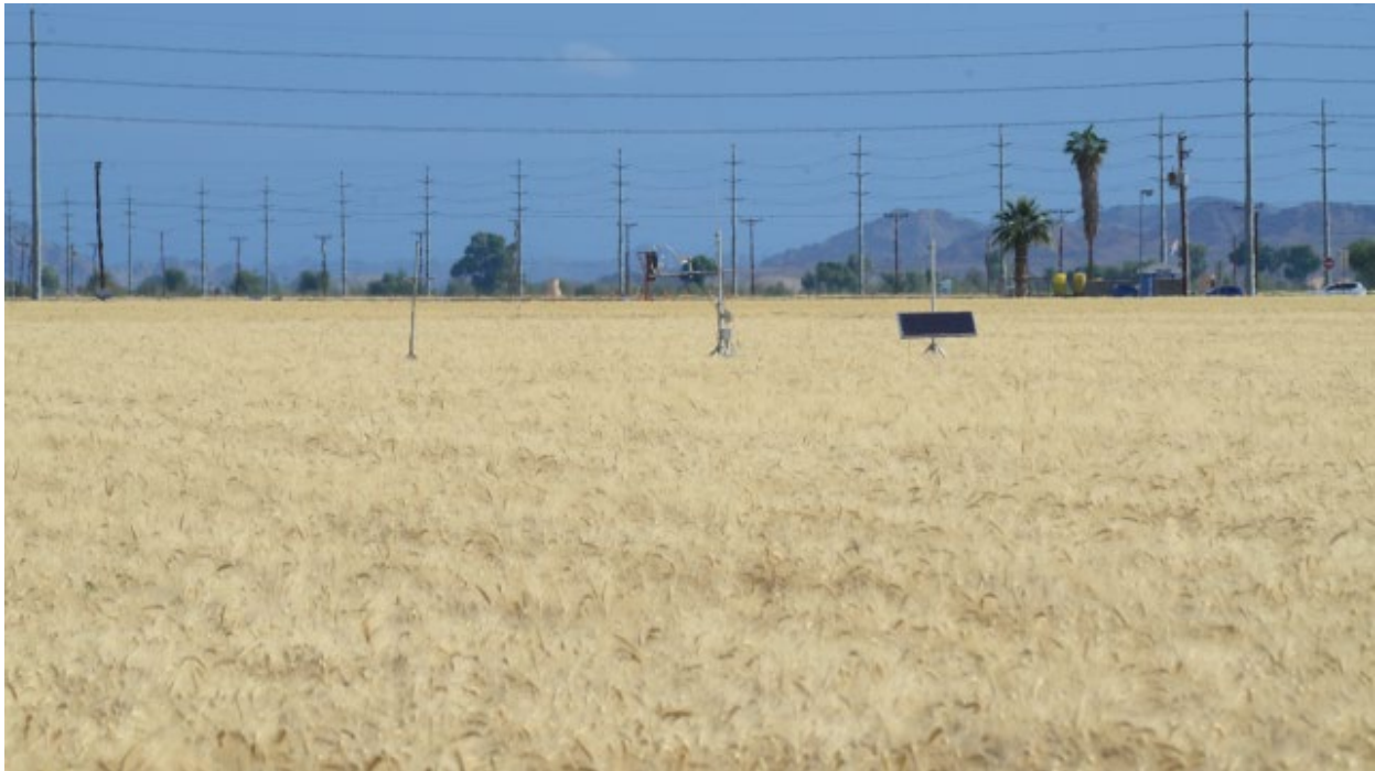
Shown are a typical deployment of three masts: net radiometer (left), eddy covariance main station (middle), and solar power supply (right).
