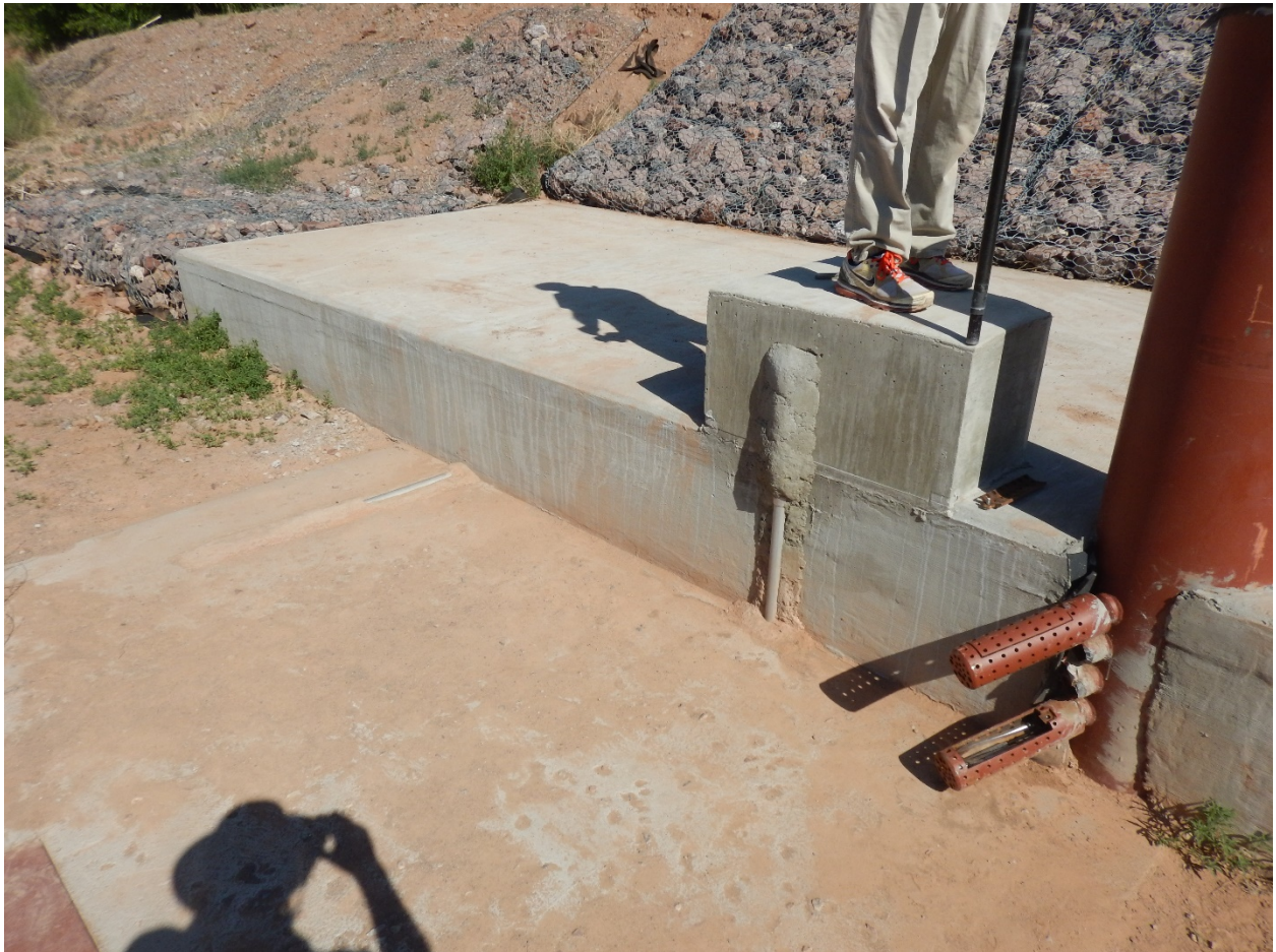
Figure AA- 3 Right bank of the sediment research station. Two perforated pipes protruding from the stilling well are each oriented downstream and house the an optical turbidimeter and the intake end of suspended sediment sampler. Two pipe microphones downstream of the stilling well (one vertical, one horizontal) are positioned in investigate the vertical concentration profile of suspended sediment. A pressure transducer is mounted inside the stilling well to measure stage during storm events.
