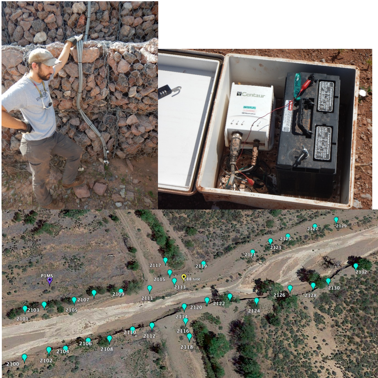
Figure AA- 10 Relevant instrument deployments at the Arroyo de los Pinos from associated researcher. Top Left: Passive acoustic hydrophones mounted on both banks as directed by Matthieu Marineau, California Water Science Center (USGS); the left bank deployment is shown with Kyle Stark, PhD student after installation. Top Right: One seismic measuring device (node) that is part of a ~30-devices array. Bottom: array of deployed seismic nodes at the site. Background image does not show the Research Station, which is located near nodes 2113 and 2114.
