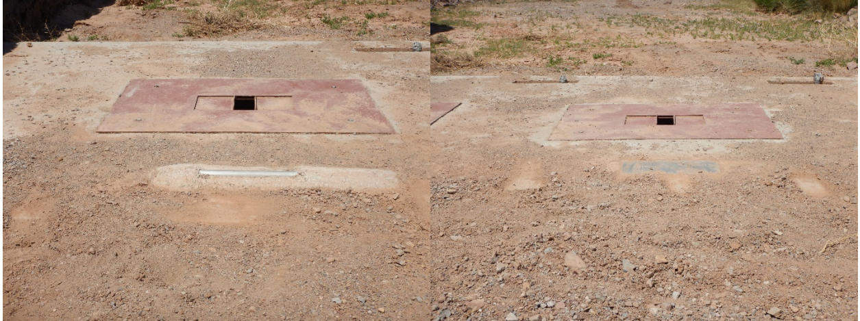
Figure AA- 2 Left: Pipe microphone upstream of Reid-type slot sampler. This is the left sampler, and right sampler is similar. Right: Plate with microphone and geophone upstream of center sampler. All slot sampler openings have adjustable widths.
