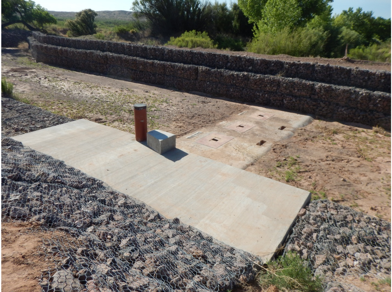
Figure AA-1 Overview of the sediment research station at the Arroyo de los Pinos. Flow direction is left to right. Concrete sill contains three Reid-type slot samplers, three active acoustic devices (two pipe microphones and one plate with microphone and geophone), and two blockouts for additional instruments. A red stilling well on the right bank contains additional instruments (see below). A concrete vault (not shown) houses the data loggers, batteries, pump samplers, and other equipment.
