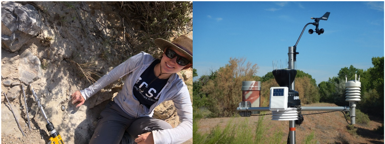
Figure AA- 7 Up-basin instrument deployment. Left: Pressure transducer to measure flow depth in an up-basin channel installed by Madeline Richards. Right: weather stations for measuring precipitation and wind speed.
