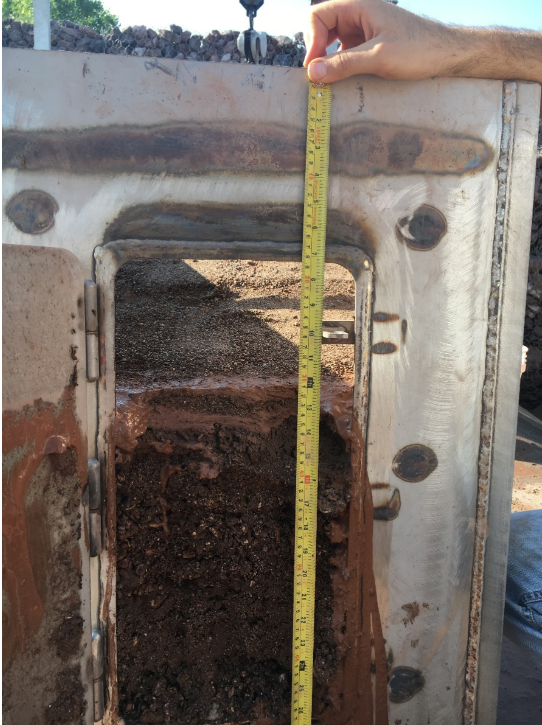
Figure AA- 5 Side door of inner metal box is open, exposing the bed load deposited during a storm event. Sediment is sampled in layers and grain size distributions are performed on each sample. After samples are collected, boxes and vaults are cleaned, boxes replaced in vault, cover is installed, and box is filled with water in preparation for next storm event.
