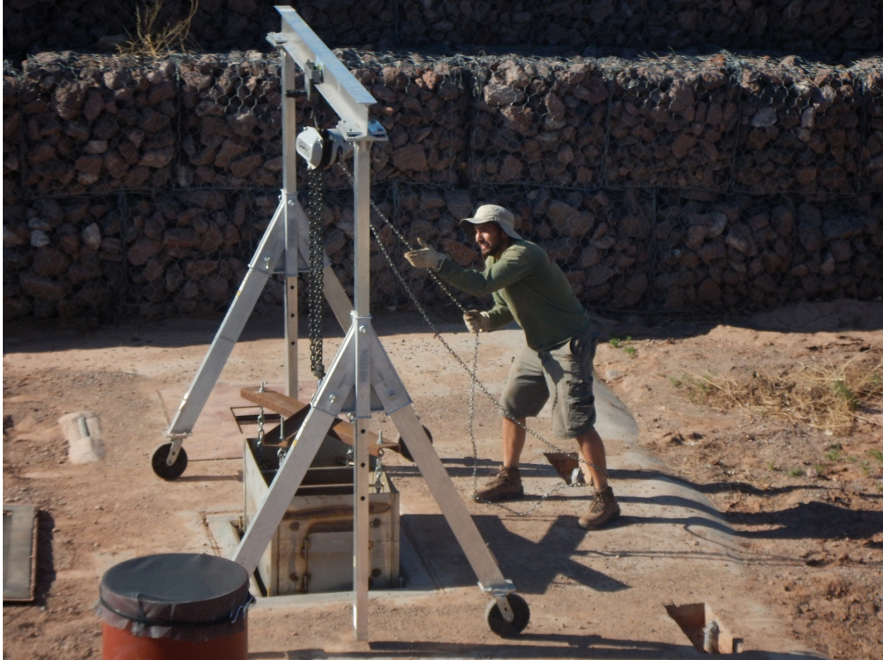
Figure AA- 4. Crane and gurney system for removing the inner metal box from the recessed concrete vault. Each metal box sits atop a pressure pillow that monitors the rate at which each box fills during a storm event. Kyle Stark operating equipment.
