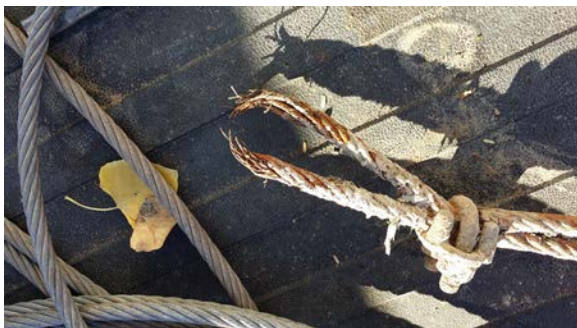
Image 3. Corrosion of log boom stranded wire anchor rope located at the Gunnison Tunnel's East Portal.
