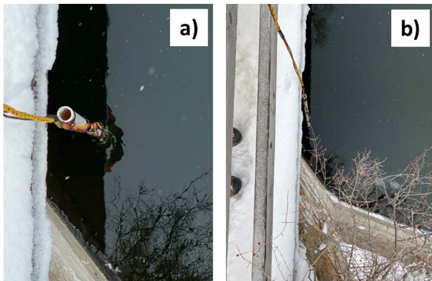
Image 6. Photo of immersed test apparatus. The temporary structure is on the submerged end of the PVC pole which was used for electrode placement and prevent excessive movement during the test.
