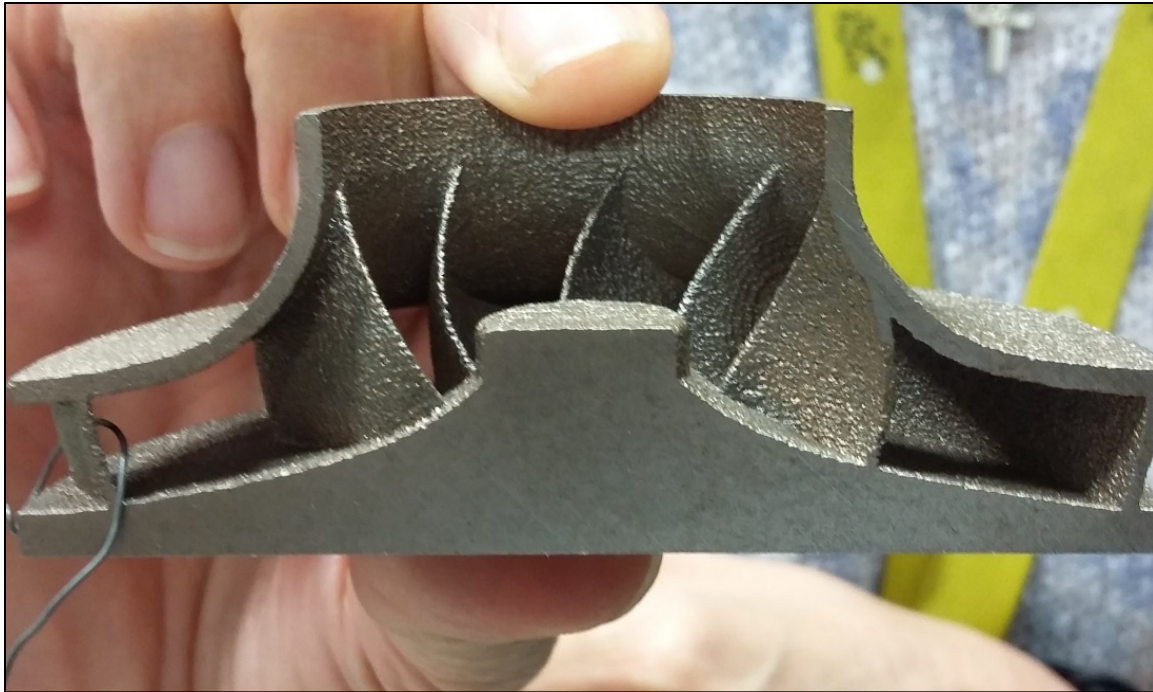
Figure ES-2.—Pump impeller printed using 3D AM technology. Note the curved impeller blades created in situ during parts creation.
