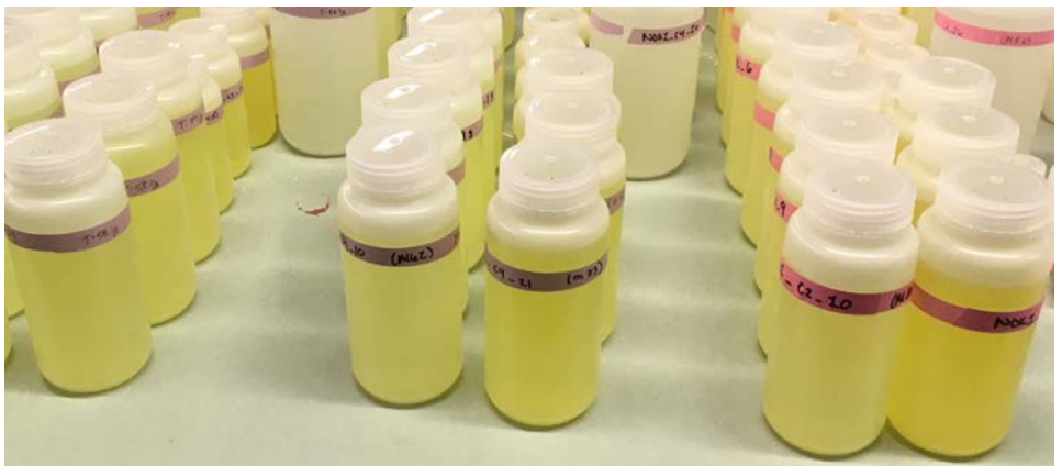
Optimization of ion exchange regeneration in TSC Reclamation facilities using different concentrations of regenerants.
