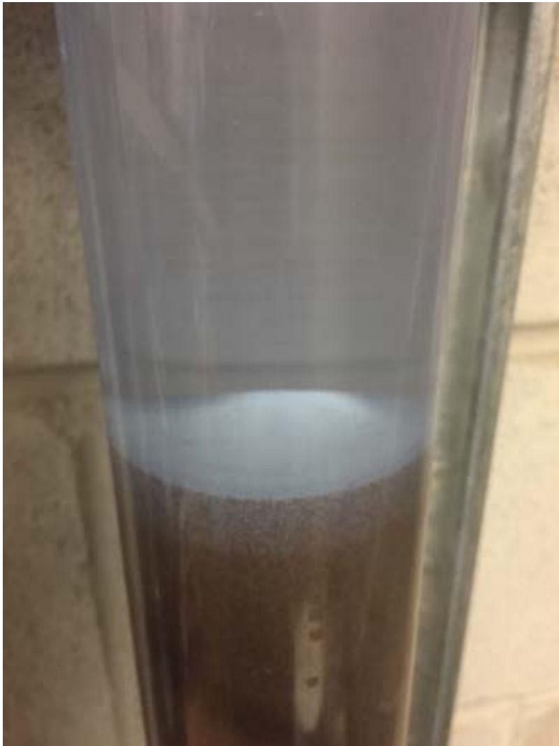
TSC Reclamation testing of stannous – chromium filtration in Norman, Oklahoma.
