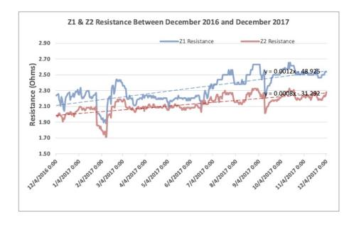
Graph of applied resistance over time indicating a decrease in moisture in the concrete.
