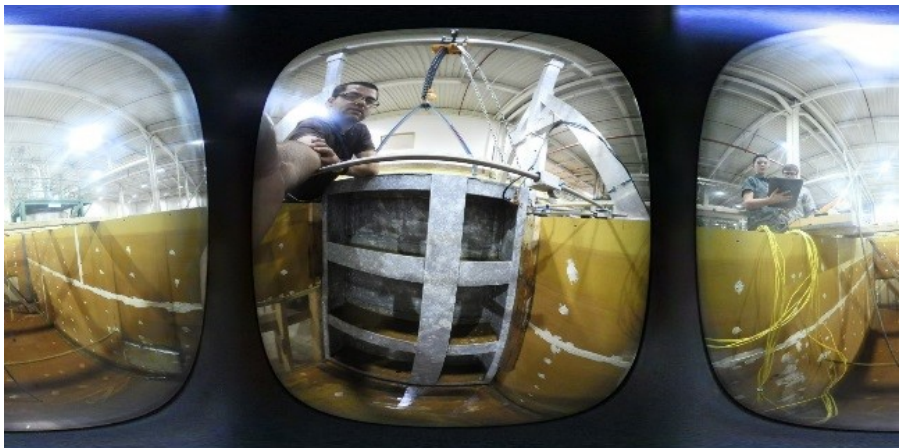
Reclamation researchers perform 360° image capture of fabricated test gate for use in photogrammetric analysis and camera evaluation.
