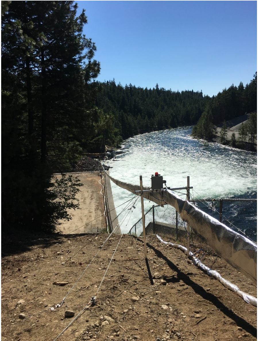
Figure 1 Whooshh™ transport tube next to Cle Elum Dam spillway, Cle Elum, Washington. Tube passed fish over the dam (1100' long and 165' high) just under an average of 60 seconds.
