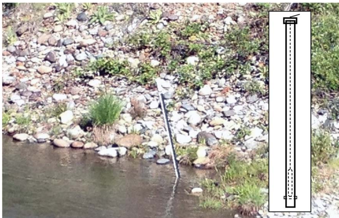
Figure 4. The downstream stage gage at Lowden. The inset white box at right shows a schematic of the stage gage design.
