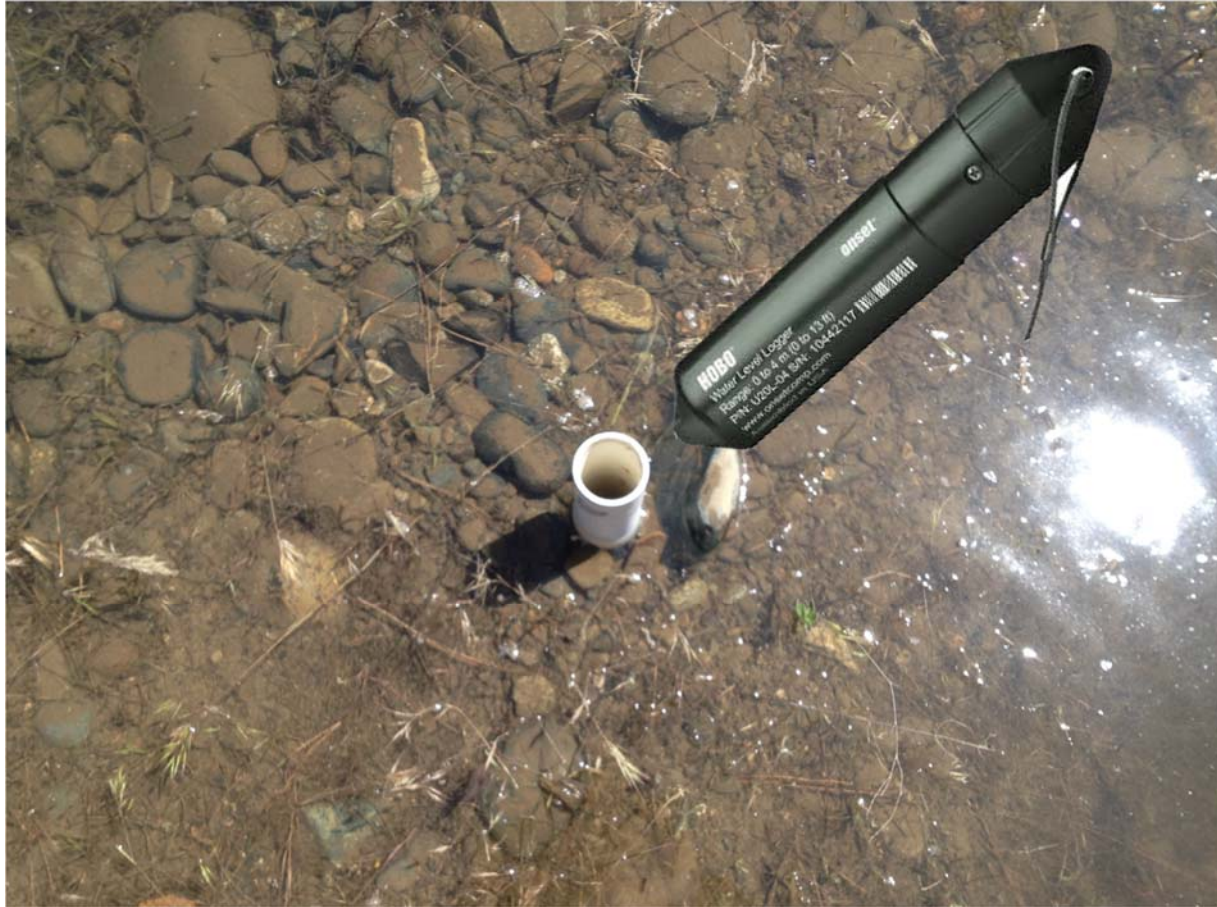
Figure 3. An uncapped well head at Lowden Ranch (center) and a picture of the Onset HOBO pressure loggers used in this study.
