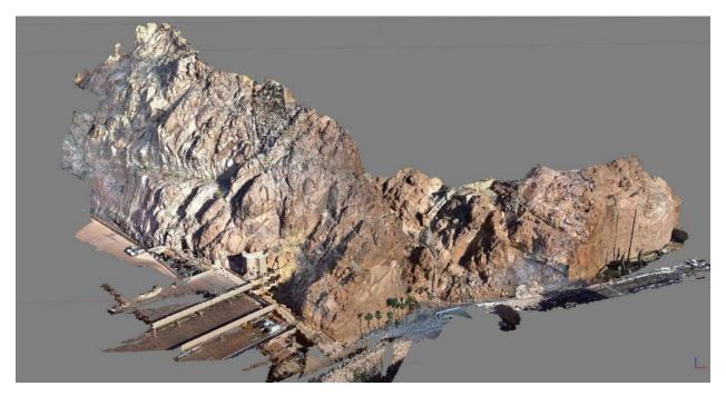
Figure 29.—Point cloud model of the rockface above the visitor center and parking garage at Hoover Dam, Nevada/Arizona.
