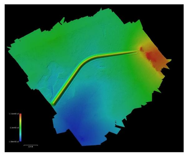
Figure 27.—Digital surface model of the left abutment of Brantley Dam, New Mexico, to investigate the use of UAS for sinkhole monitoring. Red is a higher elevation and blue is the lowest elevation.
