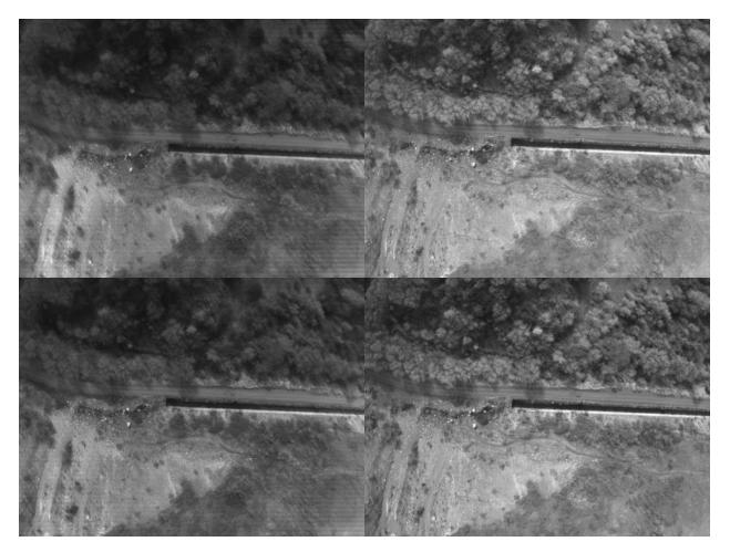
Figure 10.—The same exposure as Figure 7, but from different light bands: 550 nm (top left), 660 nm (top right), 735 nm (bottom left), and 790 nm (bottom right).
