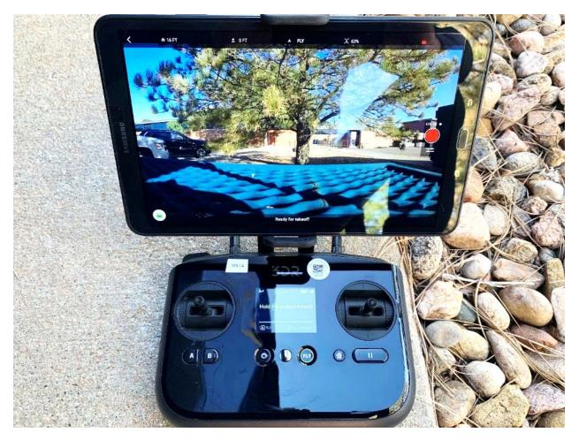
Figure 14.—3DR Solo controller with GCS. Note the flight information on the controller screen and video display on the GCS.
