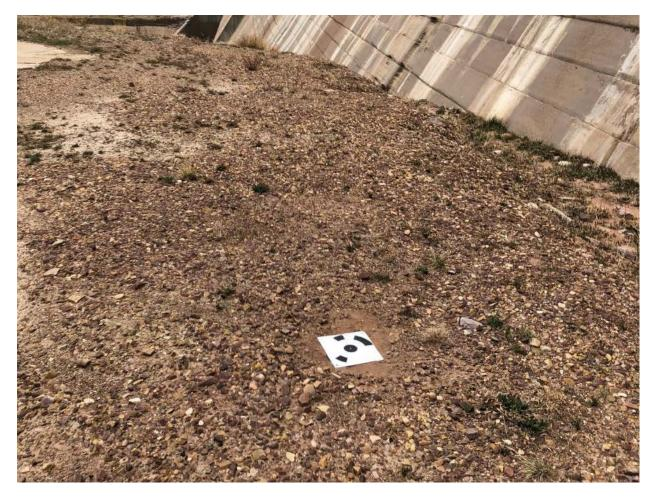
Figure 12.—Example of a coded target (Upper Stillwater Dam, Utah).
