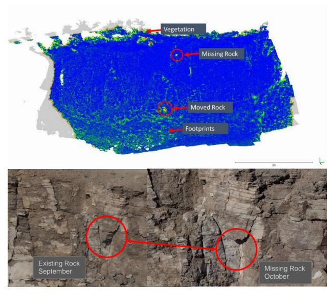
Figure 28.—Series of images showing a comparison of two models of rockface data collected a month apart, where blue shows points with no movement and red points have the most movement (top). The lower images show the rockface before and after a rock fell out of its position.
