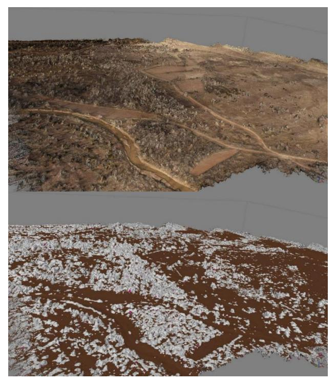
Figure 19.—Screenshots of the photogrammetric point cloud showing vegetation (top) and ground classification (bottom). The white points in the ground classification are calculated as vegetation and the brown points are estimated as ground surface.
