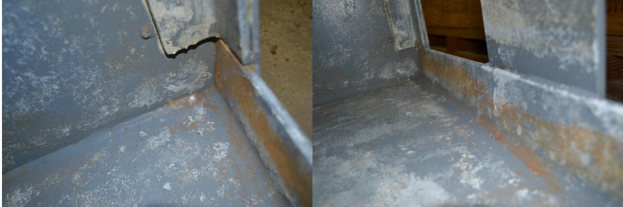
Figure 13. Photos of the front lower right corner of the test gate. Little corrosion can be seen, with most of the discoloration attributed to fouling.
