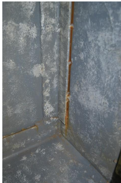
Figure 14. Photo of the back lower right corner of the test gate. Corrosion staining can be seen in the crevices that are present due to skip welding.
