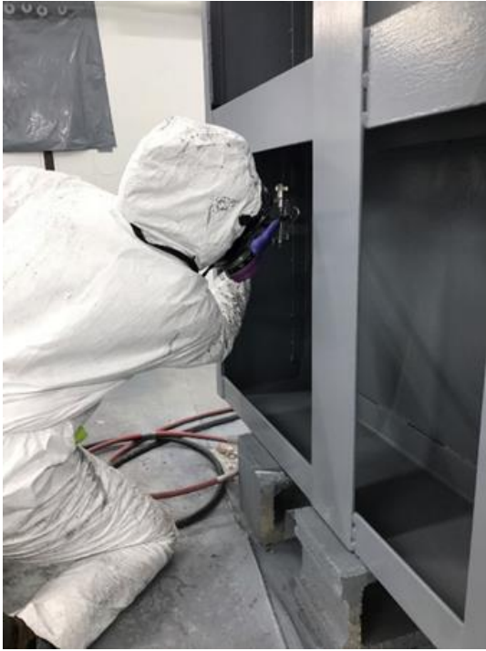
Figure 2. Vinyl coating application (left) and speckled pattern created with white topcoat (right).
