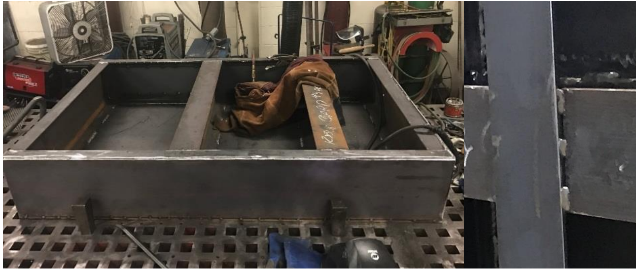
Figure 1. Bulkhead-style mild steel test gate (left) and a close-up of skip welding purposely performed to promote corrosion (right).
