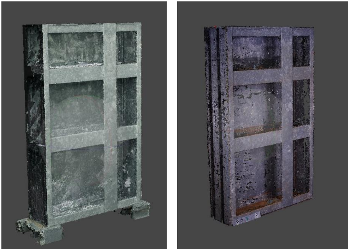
Figure 15. Isometric view of each model: uncoated, coated before immersion, and coated after immersion with corrosion highlighted in brown (from left to right).
