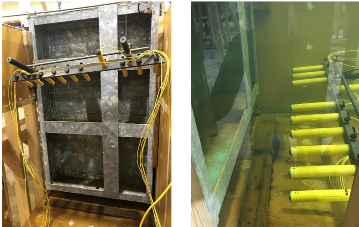
Figure 4. CSE array in dewatered test gate (left) and submerged at the bottom of flume (right).
