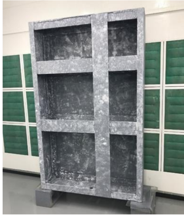
Figure 2. Vinyl coating application (left) and speckled pattern created with white topcoat (right).
