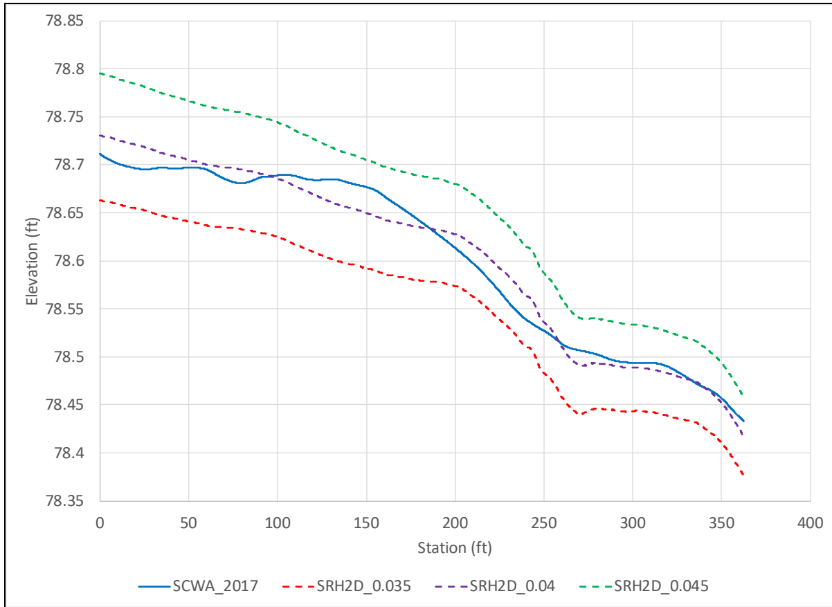
Figure 8. Model calibration to field collected water surface elevations.
