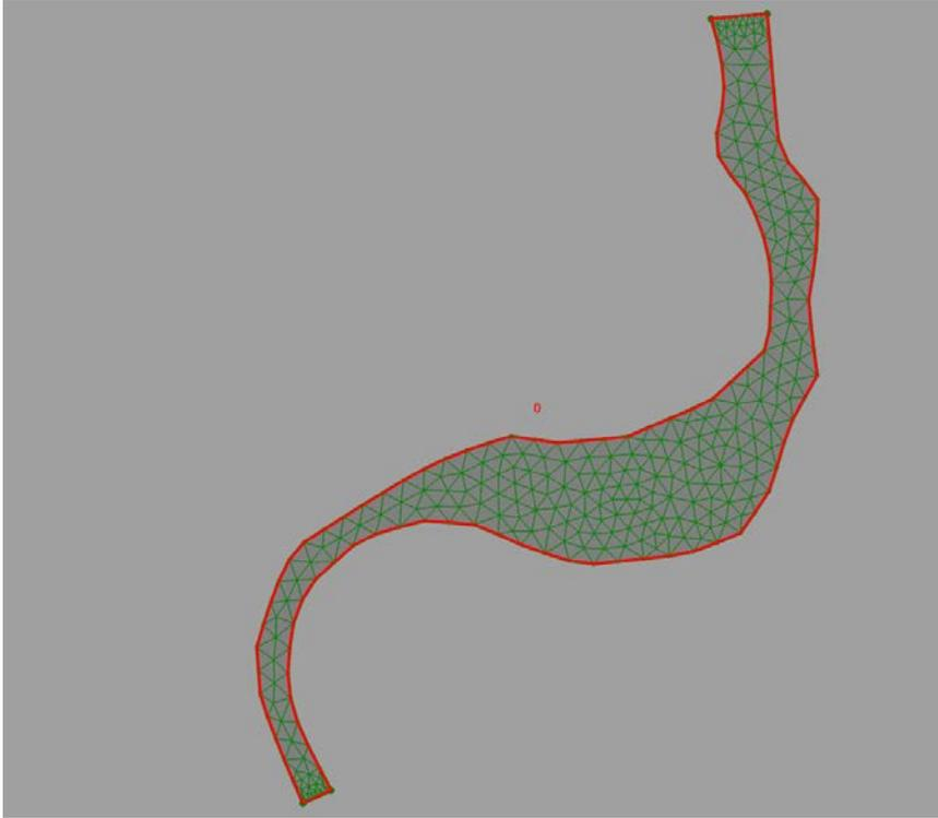
Figure 5-8. SRH-Mesh triangle mesh.
