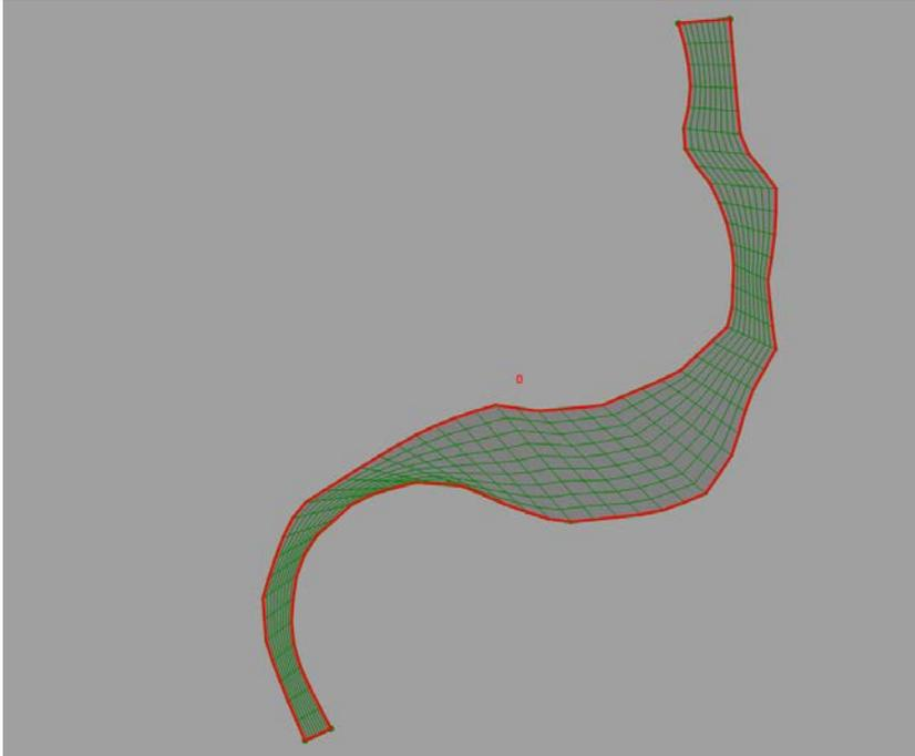
Figure 5-9. SRH-Mesh quadrilateral mesh.
