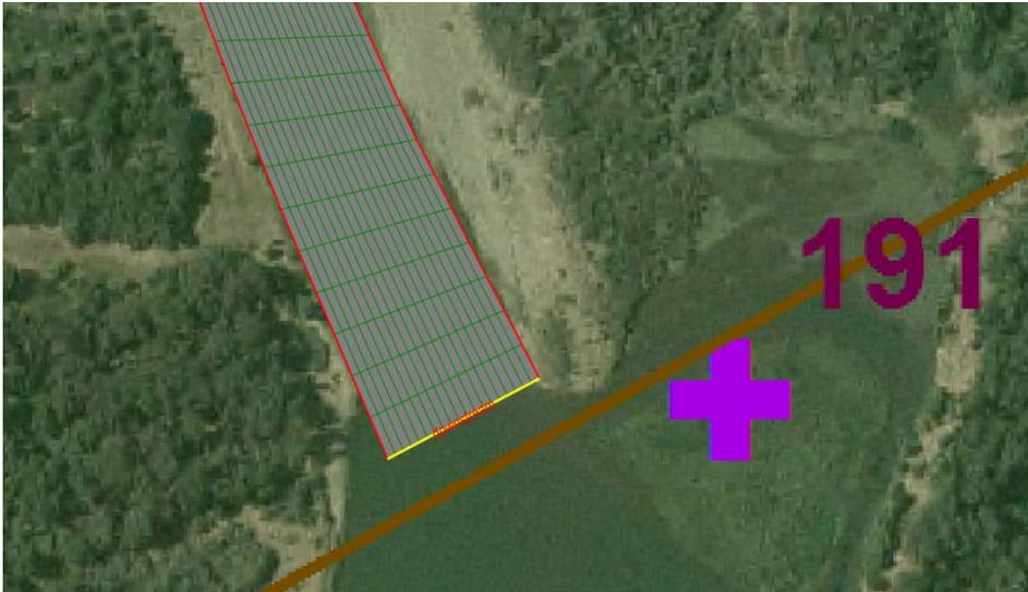
Figure 5-15. Downstream boundary condition line.
