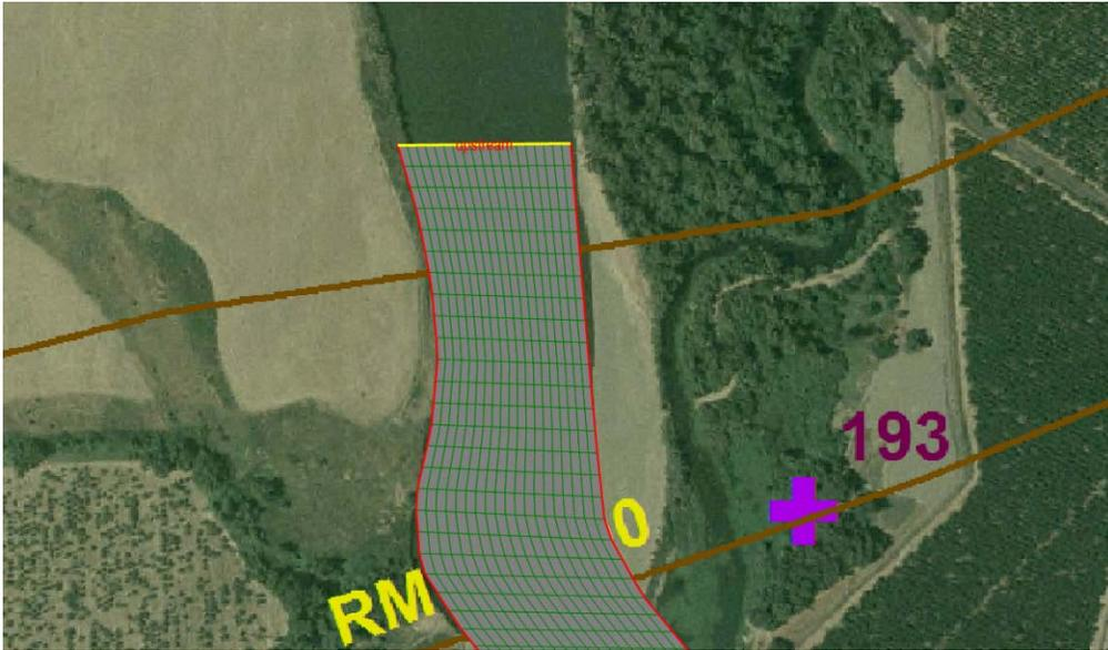
Figure 5-14. Upstream boundary condition line.
