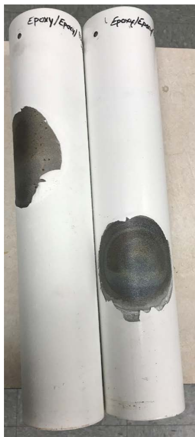
Figure 14. Cathodic disbondment of two coats of epoxy with polyurethane topcoat with and without SHDE.
