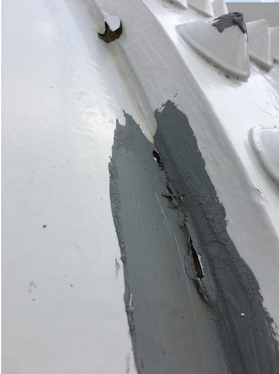
Figure 6. Anodic alkyd spot repair after 6 months the epoxy coating cracked and flaked the spot repair.
