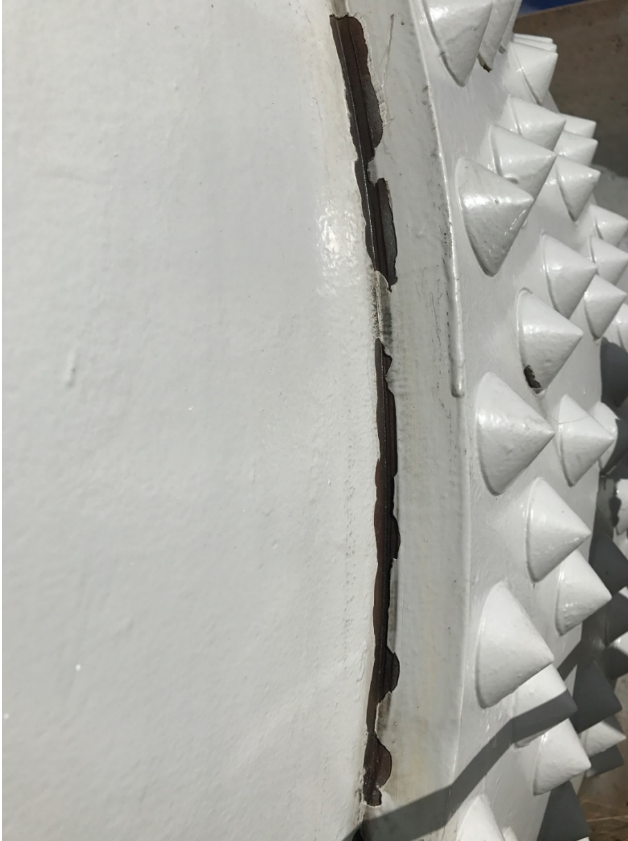
Figure 3. Appearance of steel collar/ pipe interface after surface preparation.
