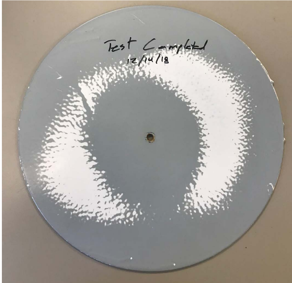
Figure 18. Erosion of Polysiloxane 2 DTM after 96hrs of slurry erosion
