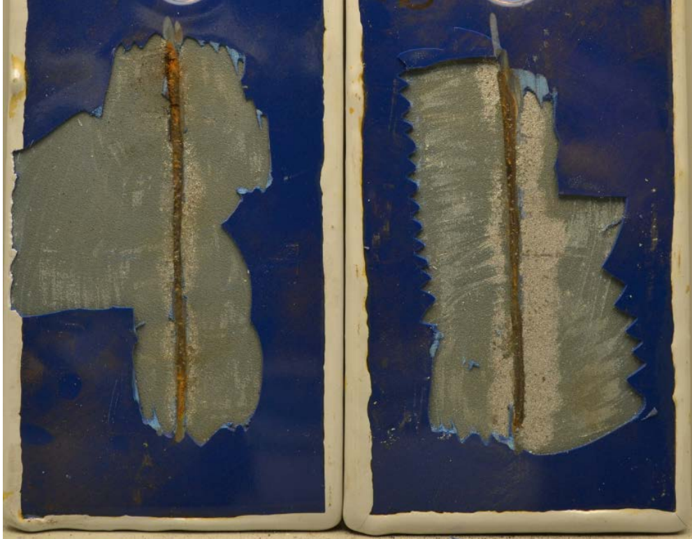
Figure 13. Flexible coating 7 wet adhesion disbondment between the zinc rich primer and the topcoat.
