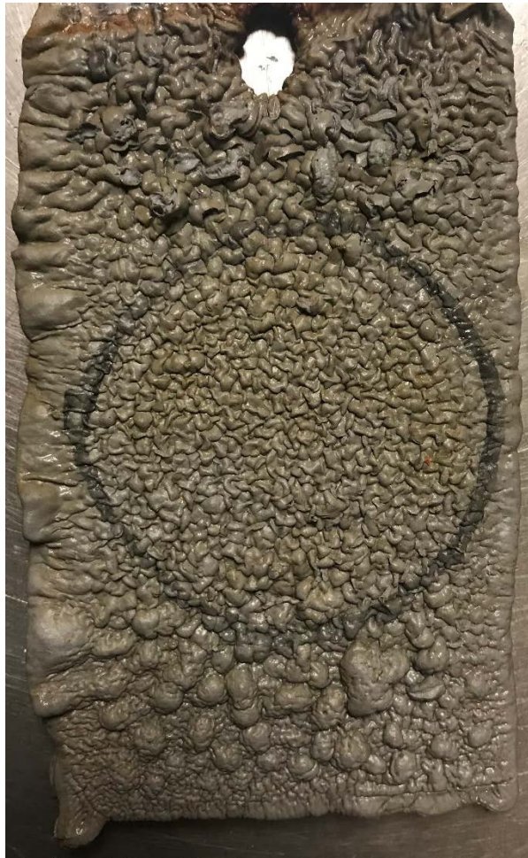
Figure 10. Failure of coating system 5, severely wrinkled in water immersion service.
