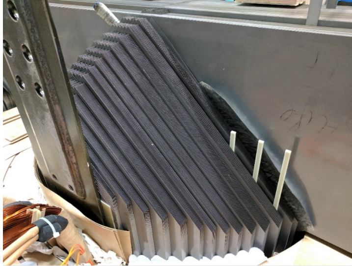
Figure 2 - Transformer Core Showing Step Laps and Cooling Channel
