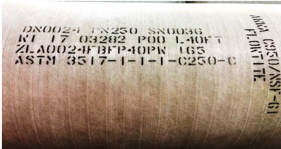
Figure A-10.—Stamping the pipe identification (diameter (24 inch or 61 cm), pressure (250 psi or 2 MPa), and stiffness (36 psi or 0.25 MPa))
