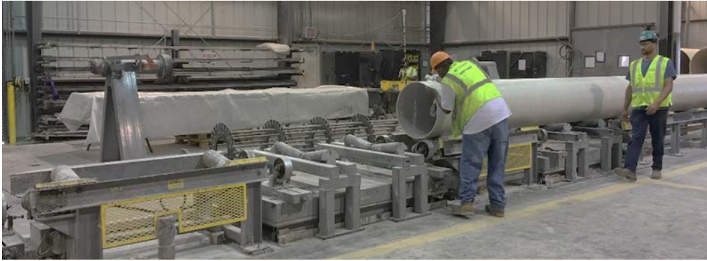
Figure A-9.—Checking the pipe and removing Mylar
