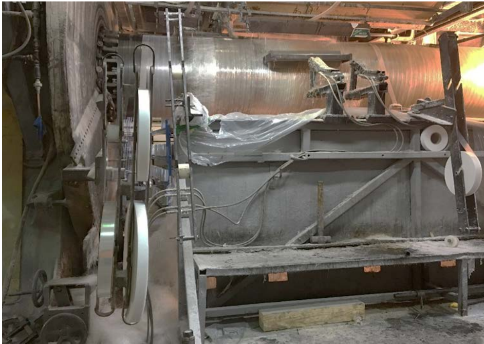
Figure A-3.—Flowtite filament wound manufacturing process
