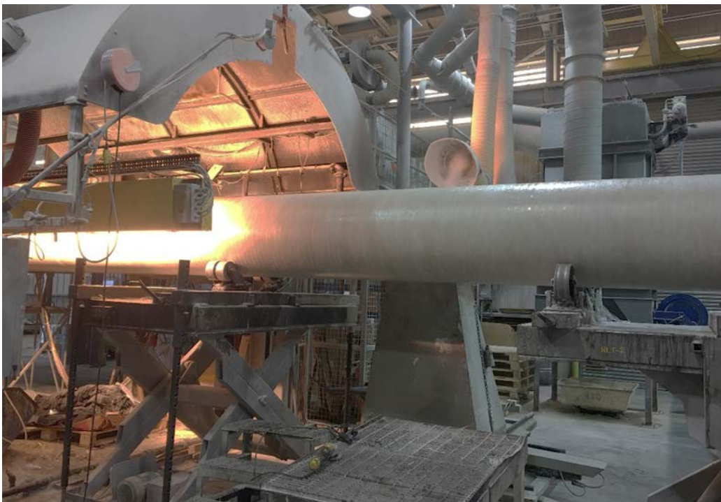
Figure A-6.—Heating system to cure resin
