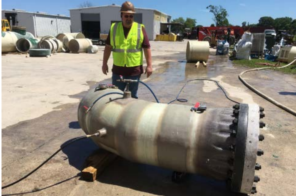
Figure A-14.—pressure testing of the fittings
