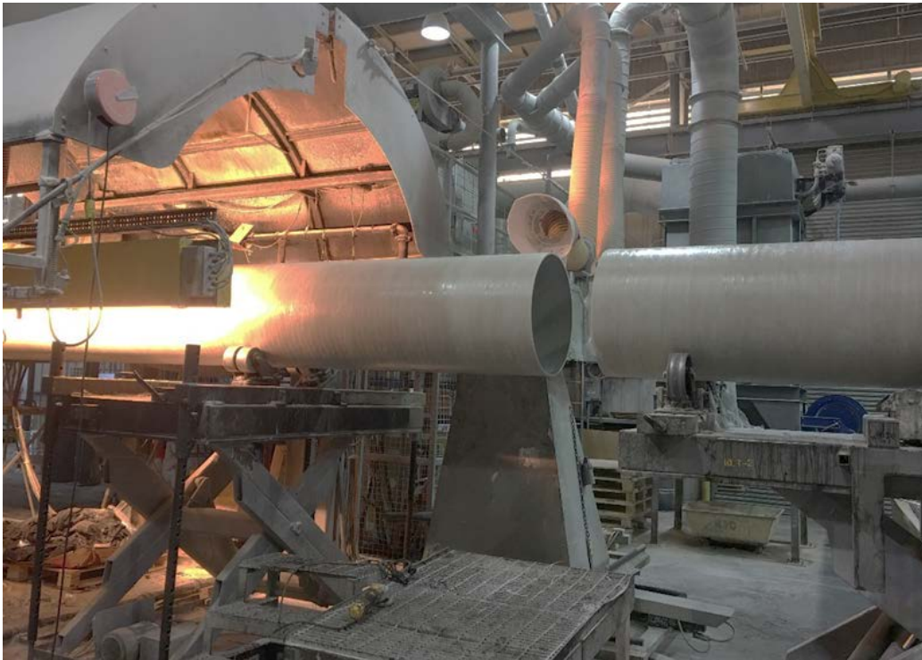
Figure A-7—Cutting pipe to the required length
