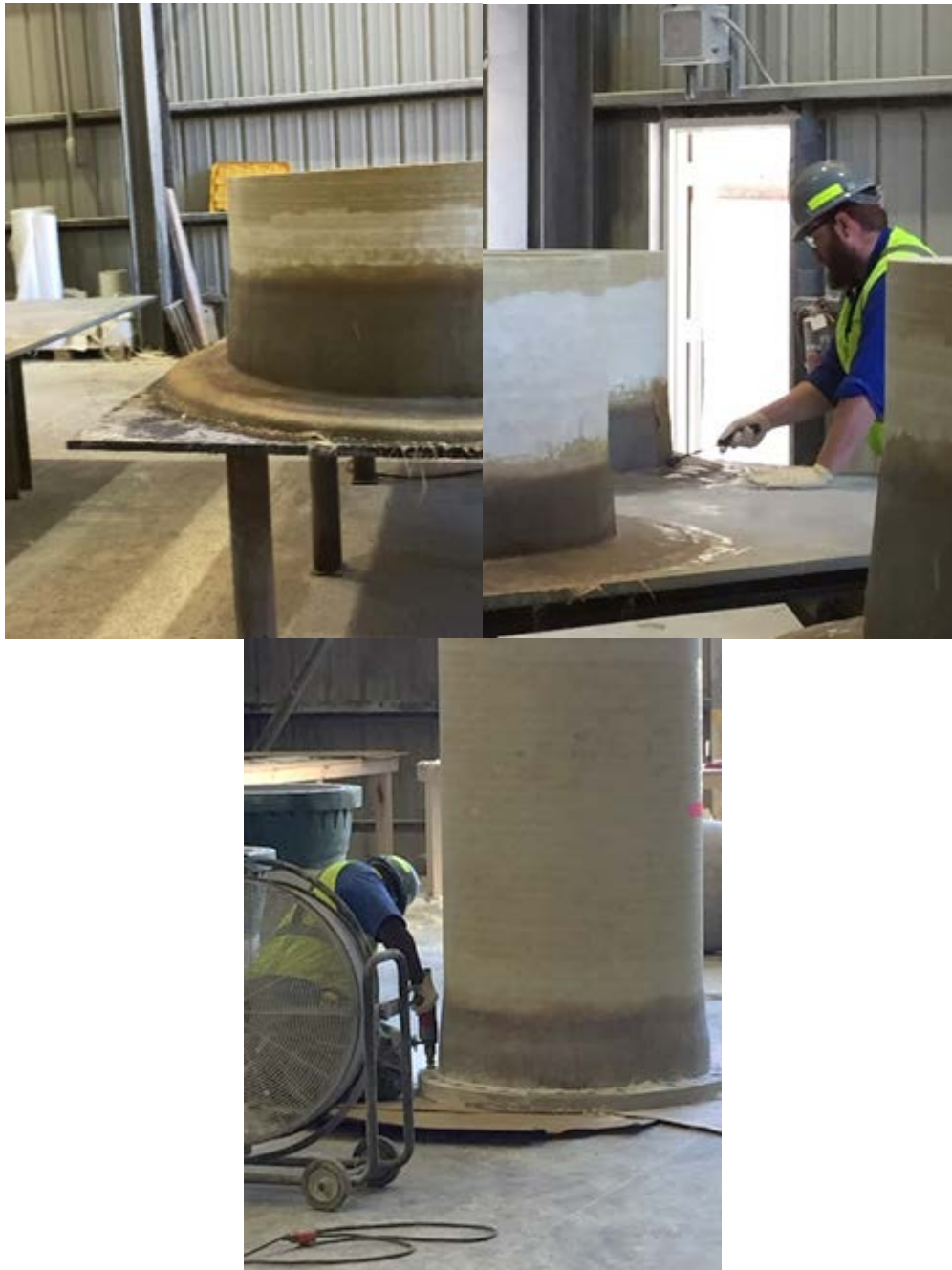
Figure A-15.—Fabrication process of flanges
