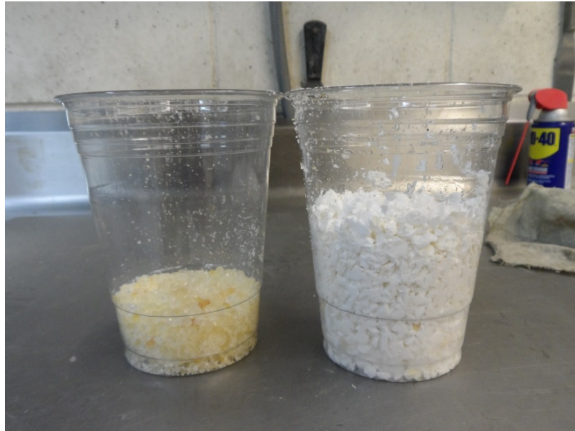
Figure 1. Ground-up Cylutions waterstop. Left side before water and right side right after water was added. The cups contained the same volume of waterstop prior to contact with water.
