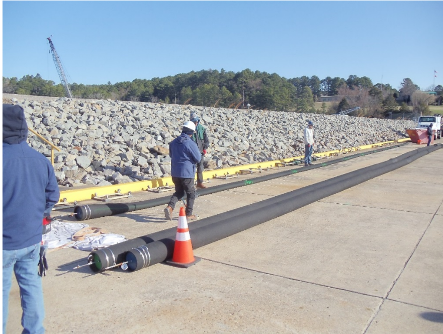
Figure 5 – View showing three waterstop membranes. The two membranes in the foreground are currently being tested with pressure. The membrane in the background is being collapsed with a vacuum.
