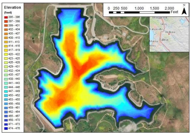
Figure 3. San Justo Reservoir bathymetric chart from 2017 survey.
