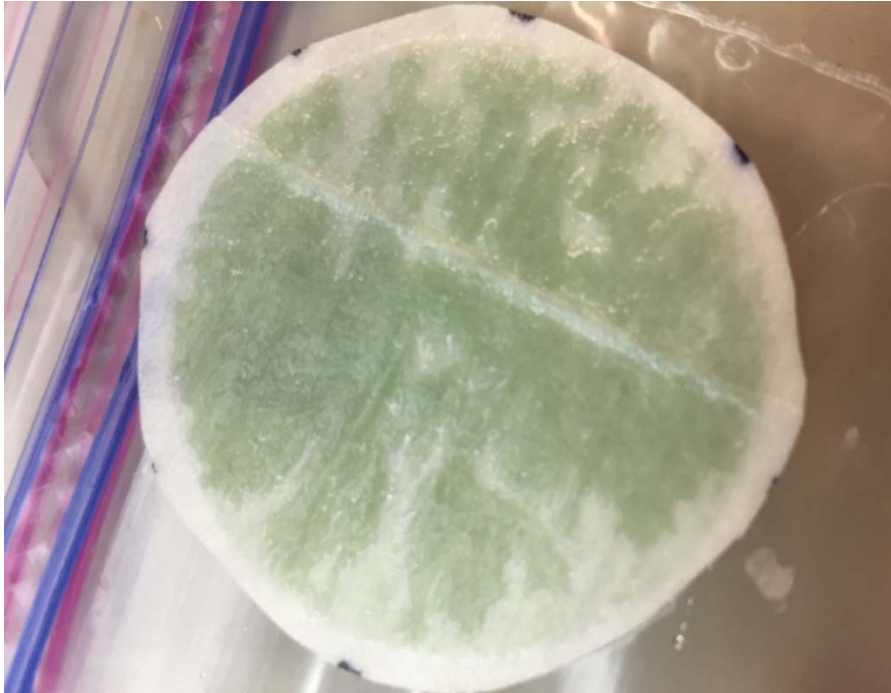
Figure B 3. Cutout of a 20 µm PCF filter after testing with OK.
