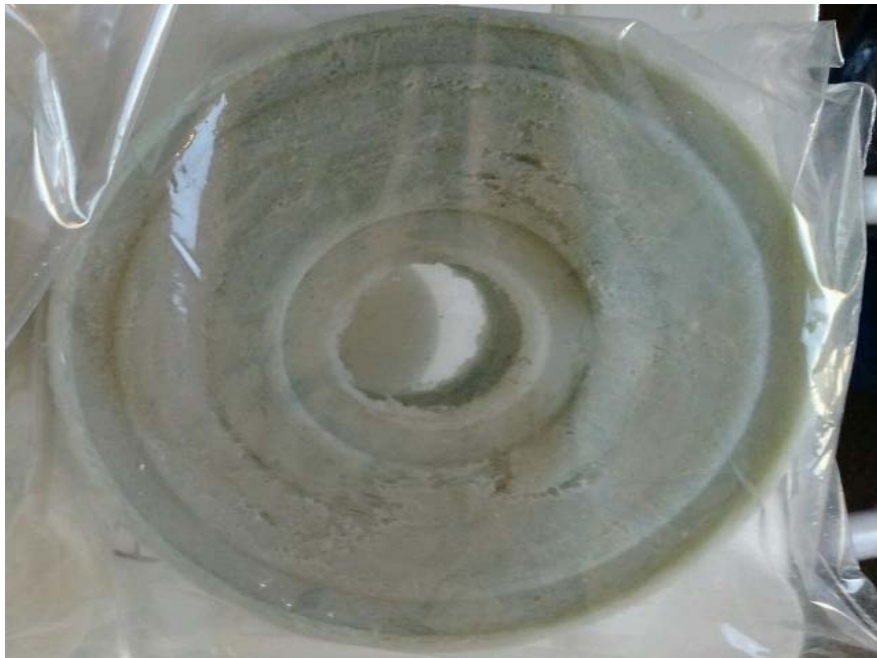
Figure B 4. Cutout of a 5 µm DCF filter after testing with CA-1.
