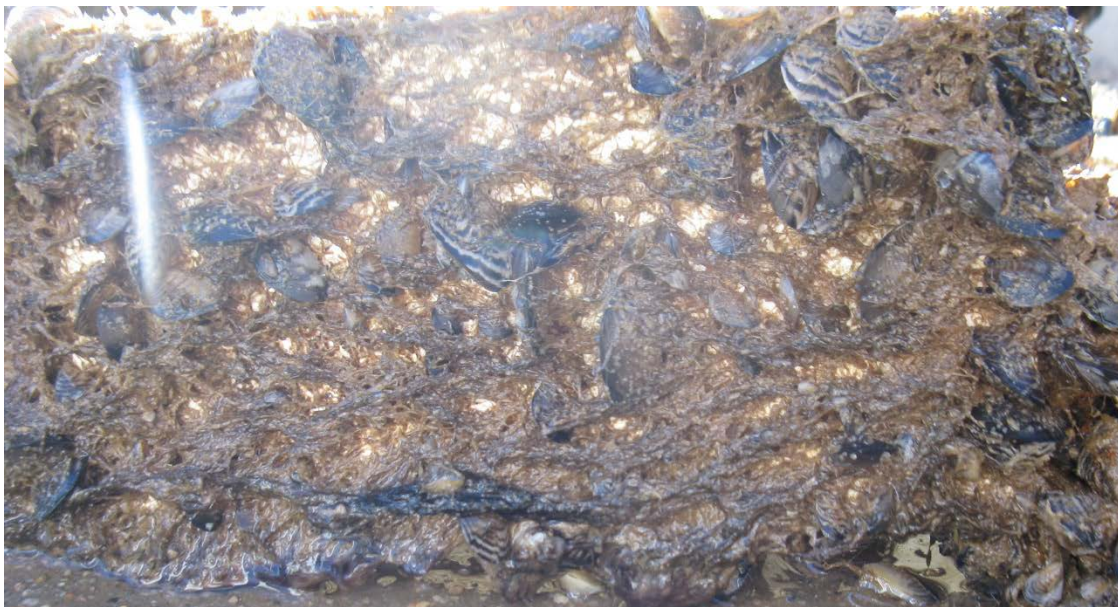
Figure 12. 15-MTA-8-2012 #1 after one year of dynamic exposure, photo taken December 2016.
