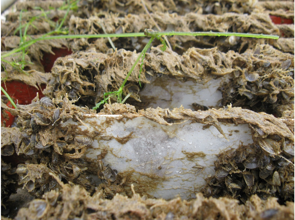
Figure 8. Partner 2012-MTA-9-1003 formulation C4-20% after three years' dynamic water exposure, photo taken July 2017.
