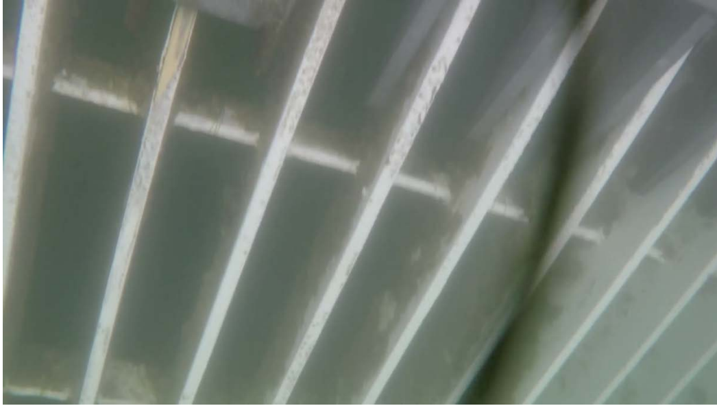
Figure 14. International Paint Intersleek 970 after 3.5 years exposure, photo taken underwater in July of 2017.
