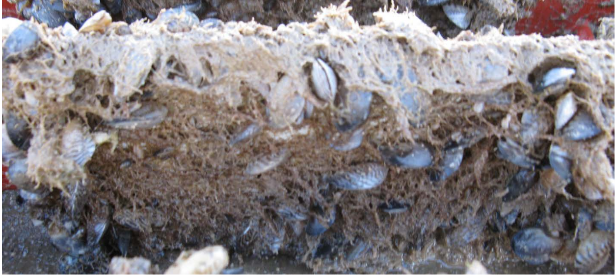
Figure 13. 15-MTA-8-1013 #1 after one year of dynamic exposure, photo taken December 2016.
