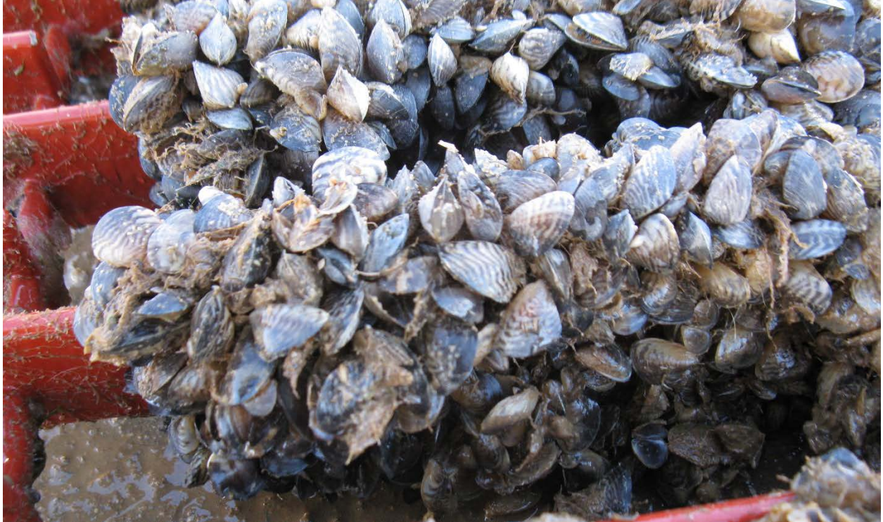
Figure 11. 14-MTA-8-1008 #1 experimental formulation after one year of dynamic exposure, photo taken December 2016.
