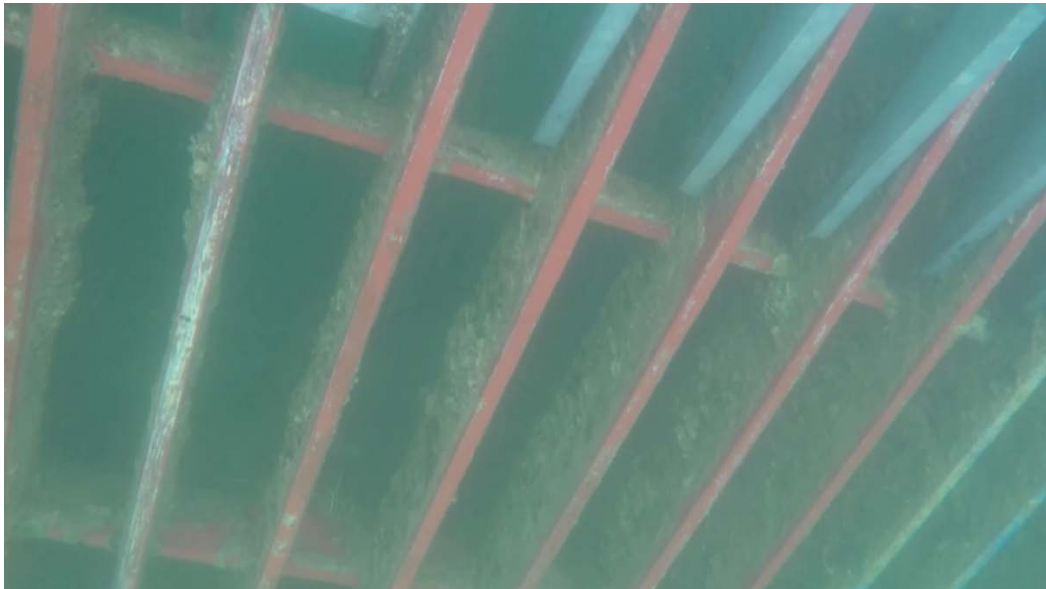
Figure 15. Sigmaglide 890 after 3.5 years exposure, photo taken underwater in July of 2017.
