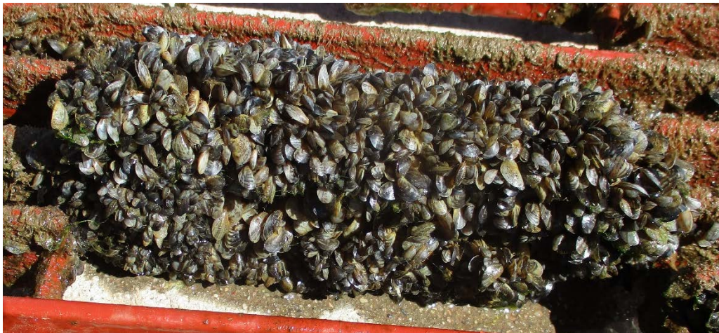
Figure 7. Sharkskin in dynamic exposure after nine months' exposure, photo taken April 2018.
