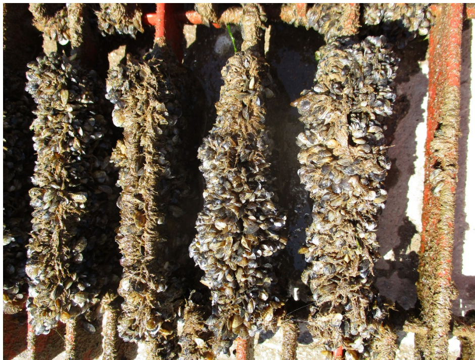
Figure 10. 14-MTA-8-1010, formulations 7, 8, 9, 10 (left to right), after 3 ½ years in dynamic exposure, photo taken April 2018.
