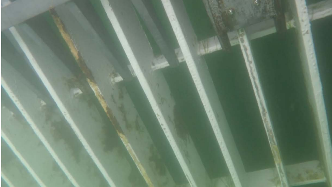
Figure 16. Sherwin Williams Sher-Release after 3.5 years exposure (no longer manufactured), photo taken underwater in July of 2017.
