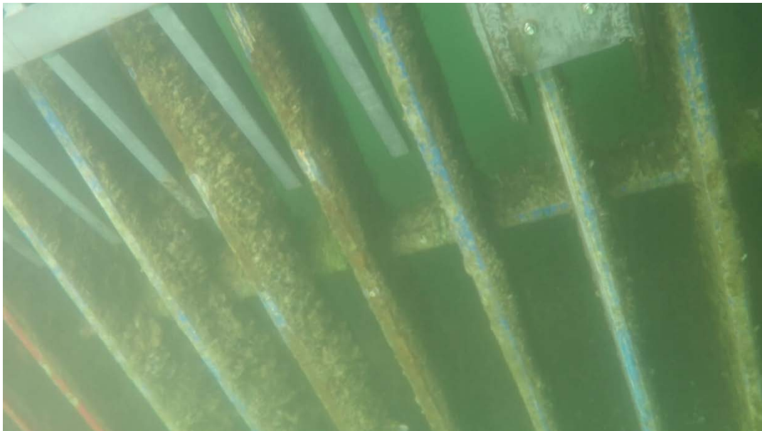
Figure 17. Seacoat Seaspeed V5 after 3.5 years exposure, photo taken underwater in July of 2017.
