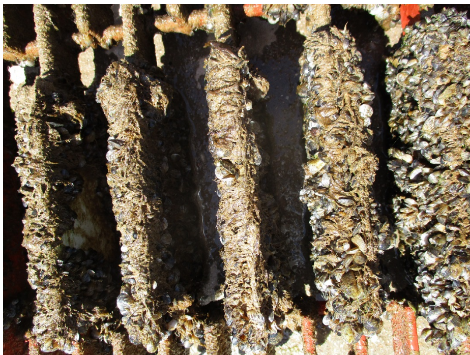
Figure 9. Partner 14-MTA-8-1010 formulations 1, 3, 4, 5, & 6 (left to right) after 3 ½ years in dynamic exposure, photo taken April 2018.
