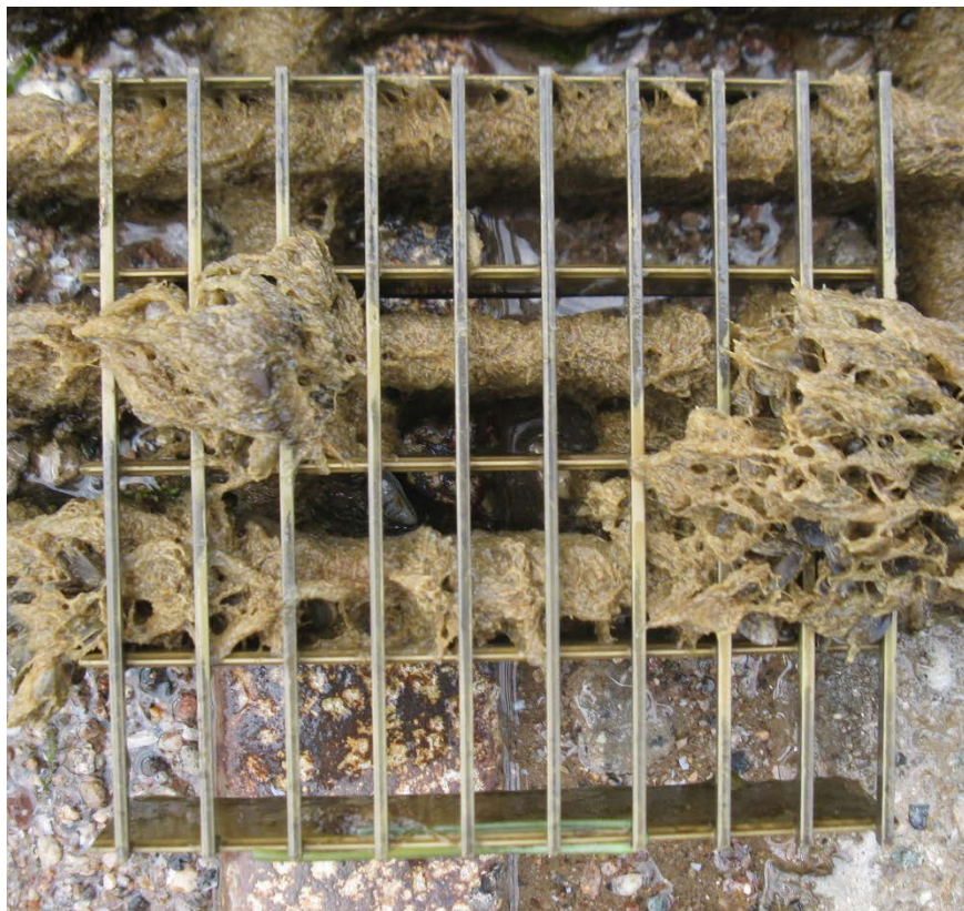
Figure 4. Z-Alloy in dynamic exposure after two years' exposure, photo taken July 2017.
