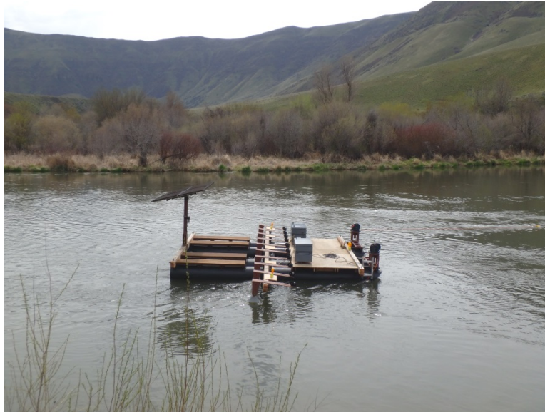
Figure 5. PIT detection barge deployed to the Yakima River fishing approximately 4,500 cfs in this photo.
