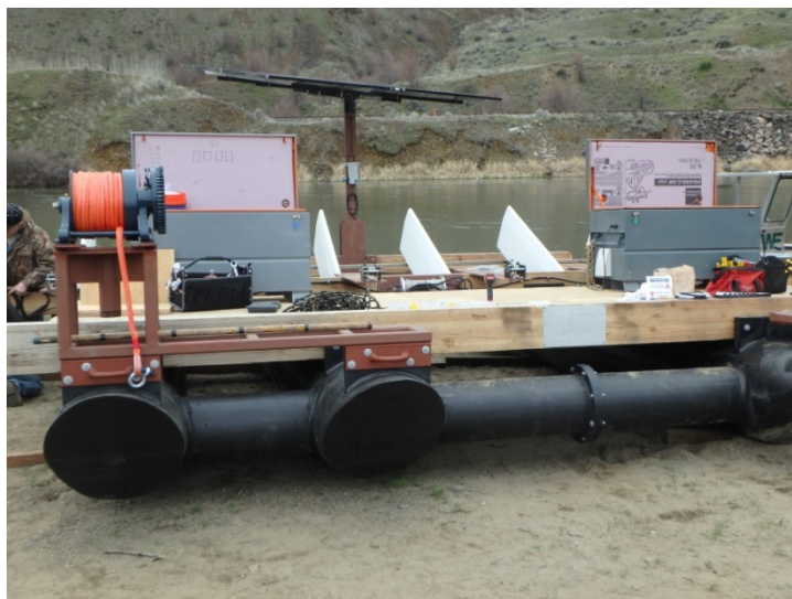
Figure 4. Integration and onshore testing of partially assembled PIT detection barge prior to launch in the Yakima River, April 5, 2017.
