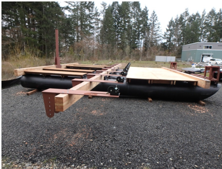
Figure 2. Assembly of barge decks and antenna, winch and solar panel bracketry fore and aft respectively.
