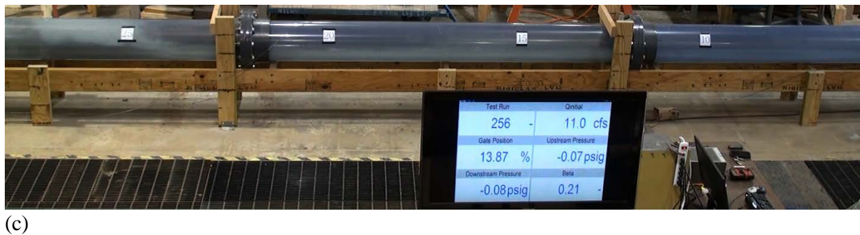
Figure 9 Time series photographs of jump motion with an undersized air vent: (a) Jump is released and begins movement (17% gate opening), (b) Jump moves downstream with air flowing back upstream (14.7% gate opening), and (c) Jump is halted again further downstream in the pipe (13.9% gate opening). Water flow and jump movement are from right to left.
