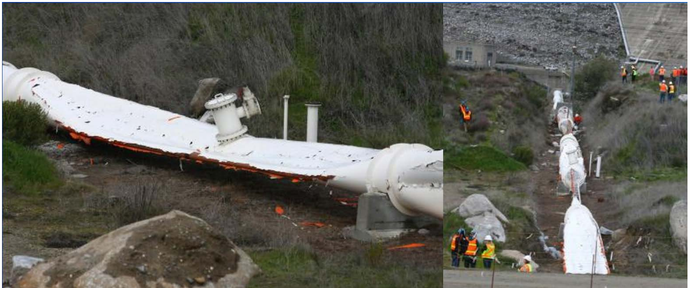
Figure 2 Example of a collapsed pipe due to negative pressures ( Link to Figure 2 photo illustrating an example of a pipe that has collapsed due to negative pressures ).
