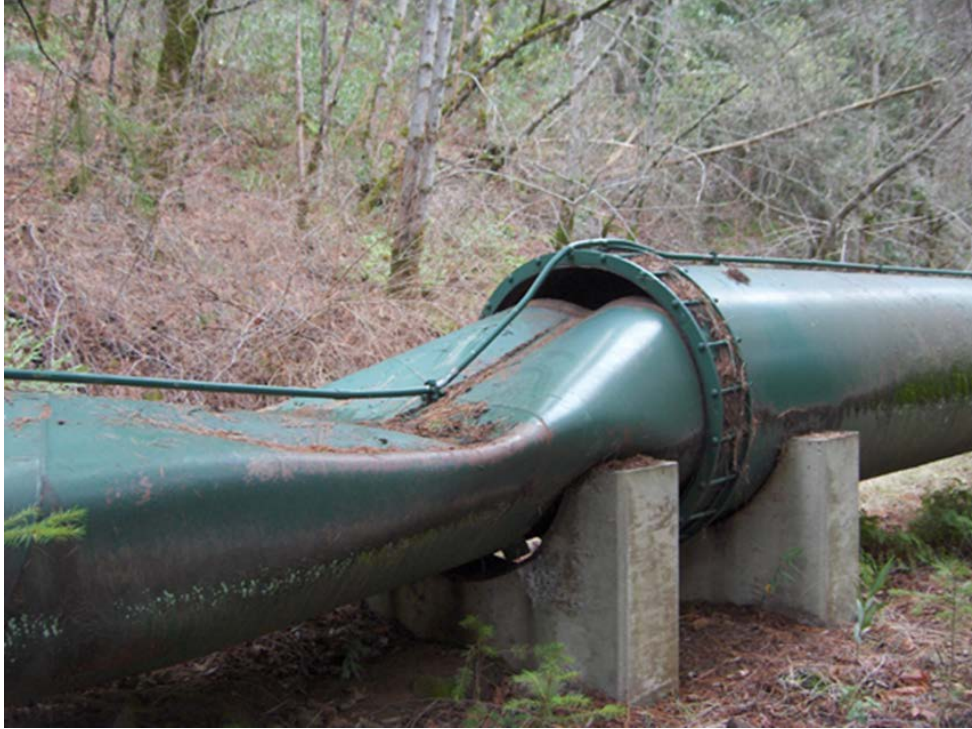
Figure 1 Example of a collapsed pipe due to negative pressure ( Link to Figure 1 photo illustrating an example of a pipe that has collapsed due to negative pressures ).
