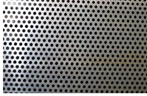
Figure 35. Perforated plate with 3/32-inch holes at 5/32-inch spacing (33% porosity).
