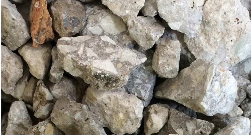
Figure 1. 2" to 4" recycled concrete aggregate used for road base
