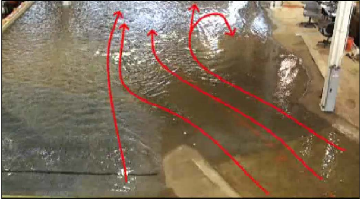
Figure 3. Manual streamlines created for the Yellowstone intake model study report (Lentz, 2014).
