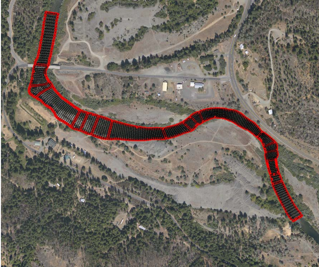
Figure 18. Model domain (red) and the mesh (black) used for the Trinity River UJC section case
