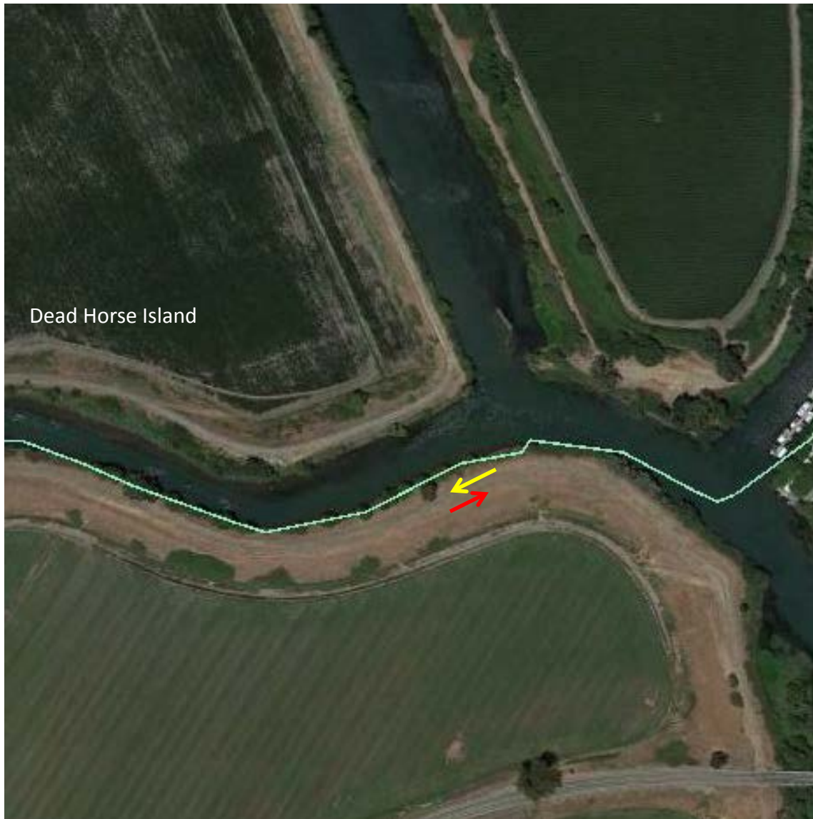
Figure 2—Locations and orientation of DIDSON camera (red arrow) and echosounder (yellow arrow) at the confluence of the Dead Horse Island Cut and the North Fork of the Mokelumne River during 2015 Delta Cross Channel data collection effort.
