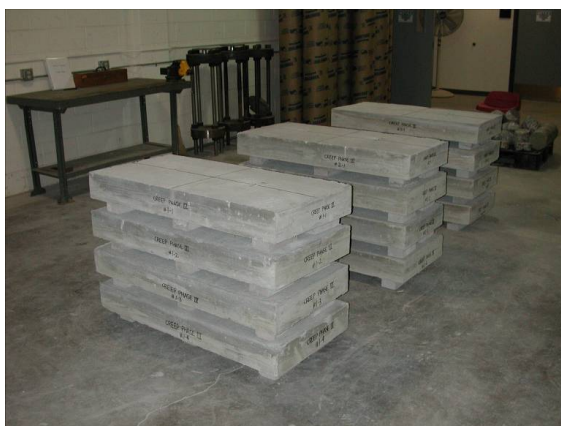
Figure 4-7: Preparation of test slabs (USBR program)
