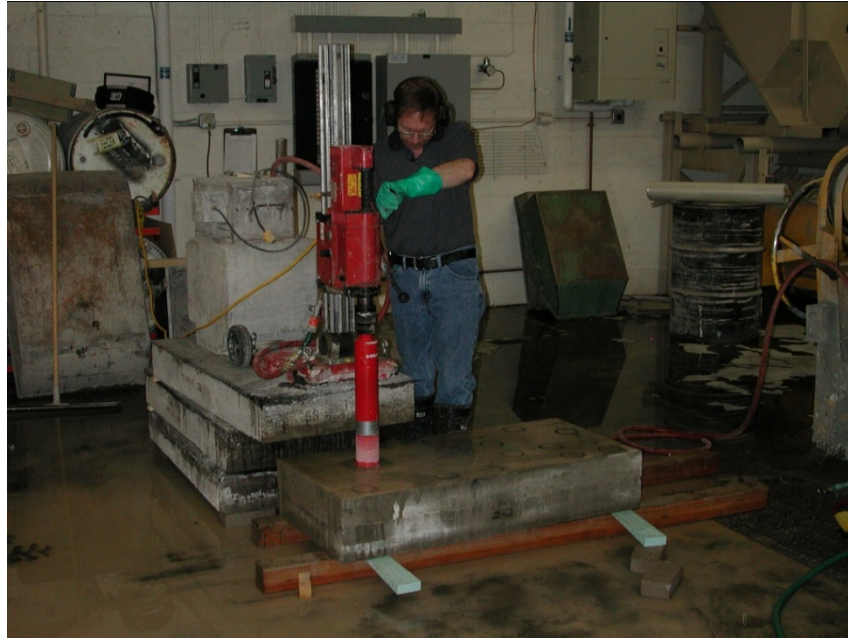
Figure 4-10: Experimental setup for coring under controlled inclination (USBR program)
