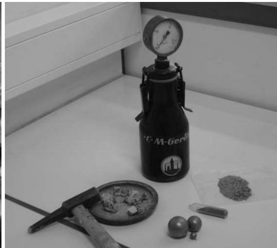
Figure 5-5: Carbide bomb test
