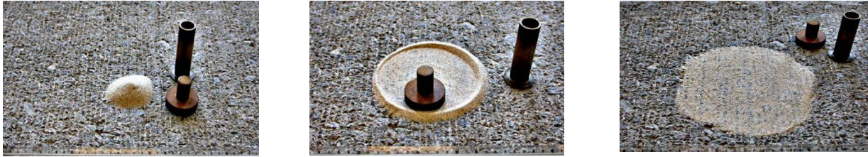
Figure 2-1: Measurement of surface macrotexture with the sand patch test procedure
