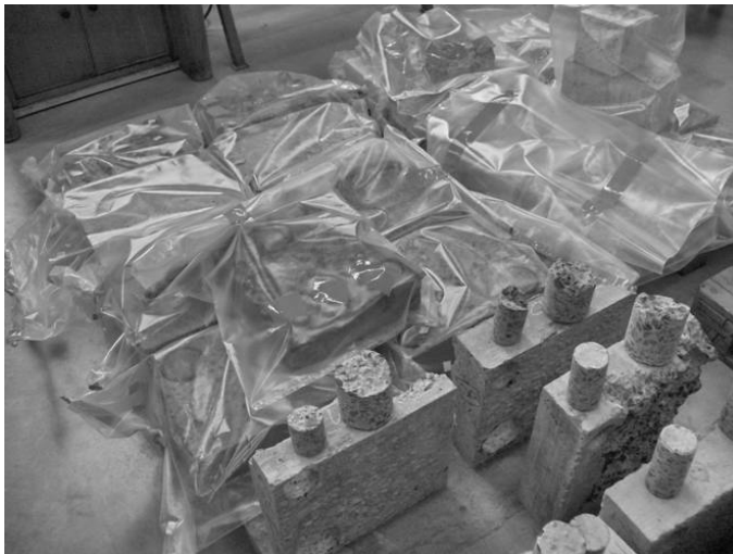
Figure 5-4: Specimen storage layout for moisture pre-conditioning
