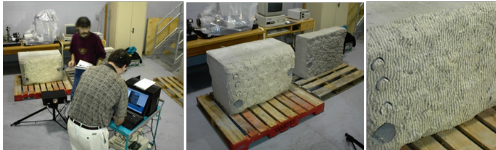
Figure 2-9: Use of an interferometric measuring device for concrete surface characterization
