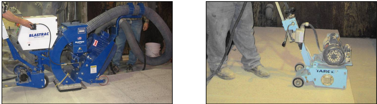
Figure 3-5: Scarification and shotblasting surface preparation at CRIB (UL program)
