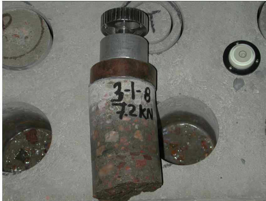
Figure 4-18: Example of an extracted core specimen drilled with a 4° angle
