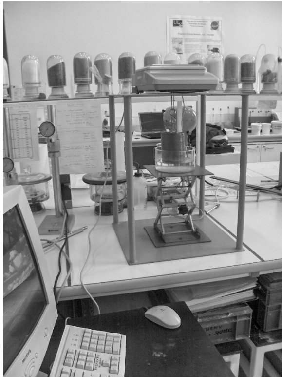
Figure 5-3: MCST testing – a) experimental setup; b) test specimen
