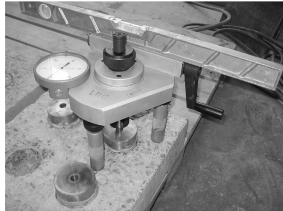
d) Positioning of the pull-off test device
