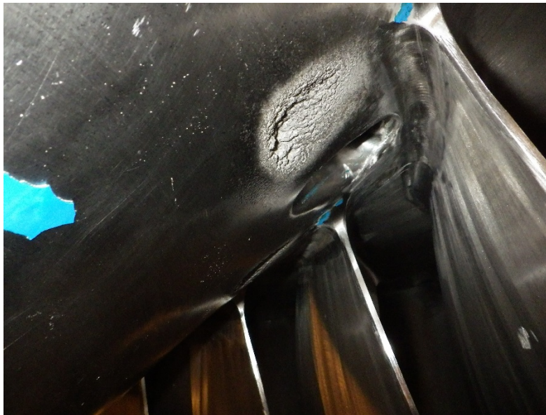
Figure 5. Additional cavitation damage downstream of the turbine air vent at Flaming Gorge powerplant.
