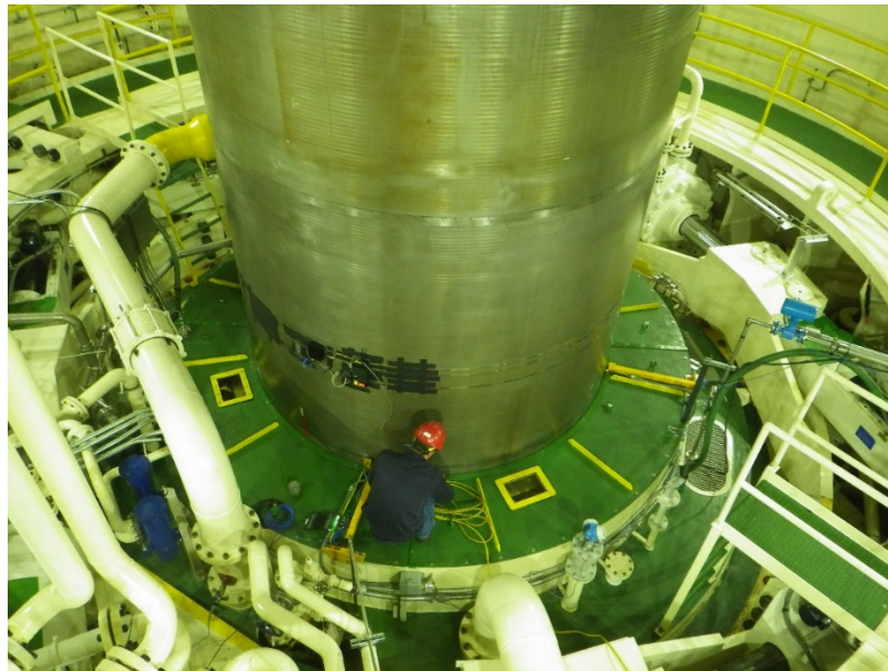
Figure 7. Grand Coulee Unit G24 turbine shaft with attached AE sensor and accelerometer, and wireless data transfer system.
