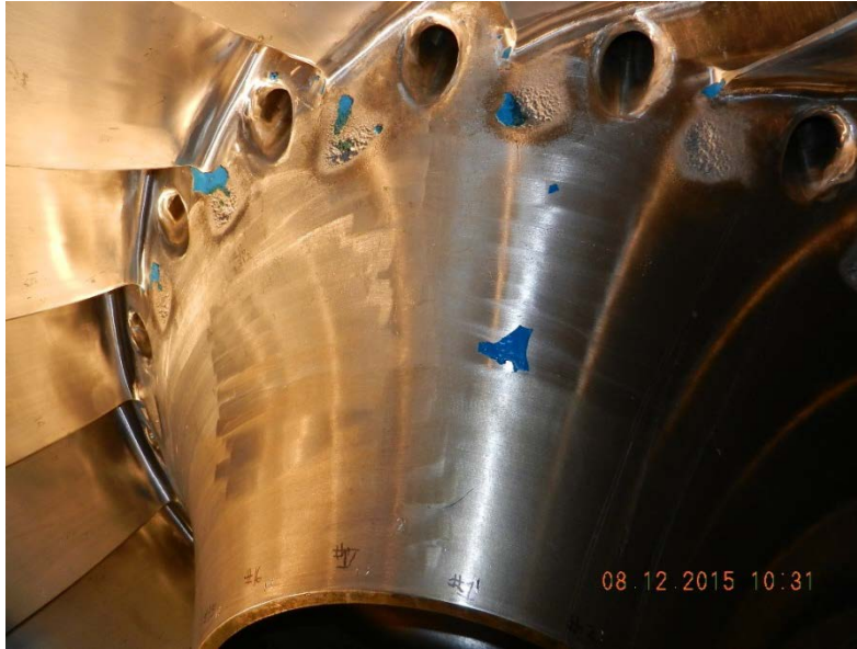
Figure 4. Typical cavitation damage downstream of the turbine runner air vent at Flaming Gorge powerplant.
