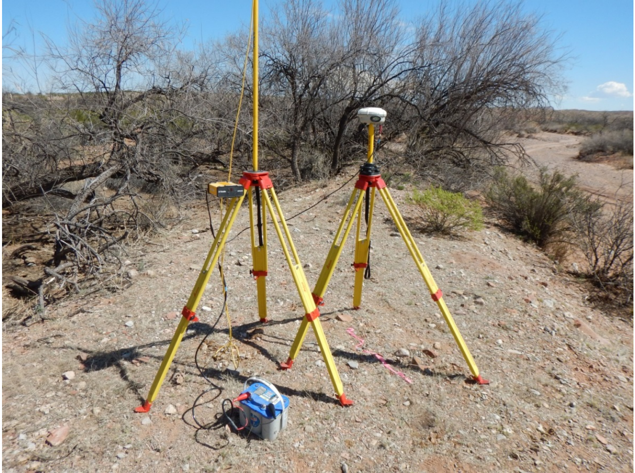
Figure 2. Base station set up over the control point for the RTK-GPS survey. Cap on control point is stamped "Pinos 1" and is located directly under the Trimble R8 receiver (pink flagging tied around rebar).
