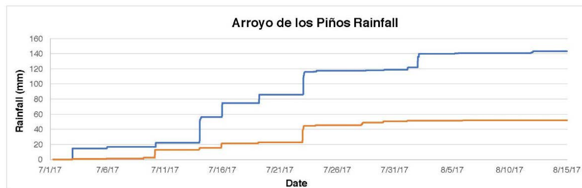
Figure D 13 Rainfall recorded in the Arroyo de los Piños watershed. Blue is the site rain gauge, near the basin outlet. Orange is the up- basin rain gauge located in the headwaters of the watershed.
