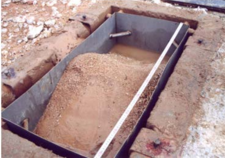
Figure A 3: Example of sampling stainless steel box sitting inside of concrete box (Varyu)
