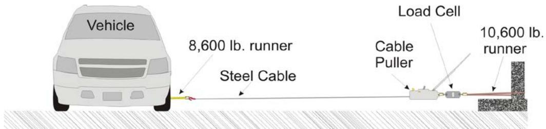
Figure 2.—Schematic diagram of typical 2009 Reclamation static vehicle anchor testing.
