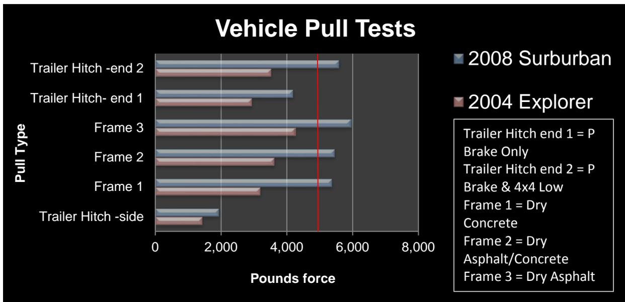
Figure 4.—Vehicle static pull testing results from March 2009 for various rigging configurations.
