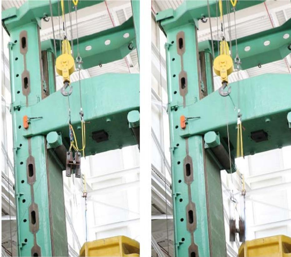
Figure 11.—Drop testing setup pre-drop (left) and post-drop (right).
