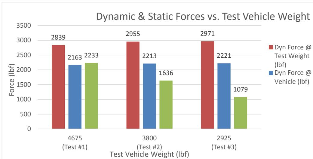
**Figure 13.—Average dynamic and static forces for three test setups.**
