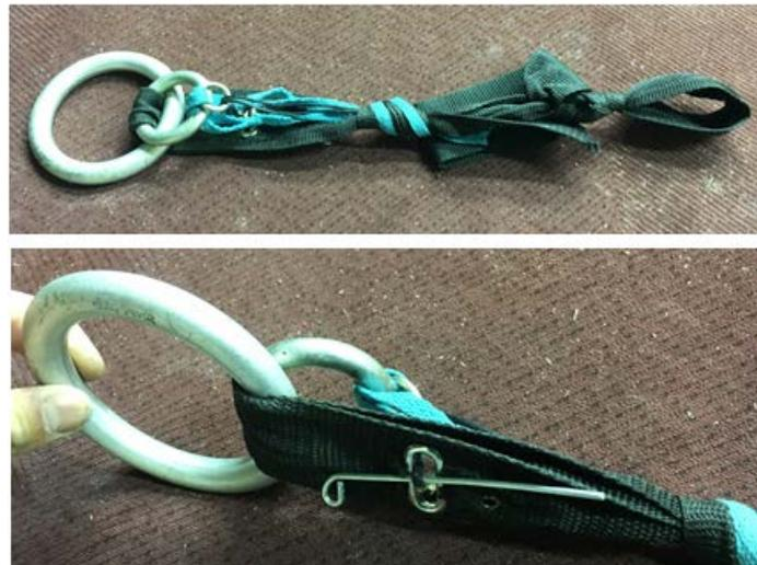
Figure 10.—Quick-release mechanism as a 3-ring release.
