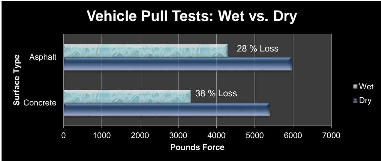
Figure 5.—Vehicle static pull testing results from March 2009 for wet versus dry conditions.
