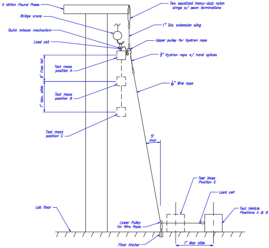
Figure 6.—Drop testing schematic.
