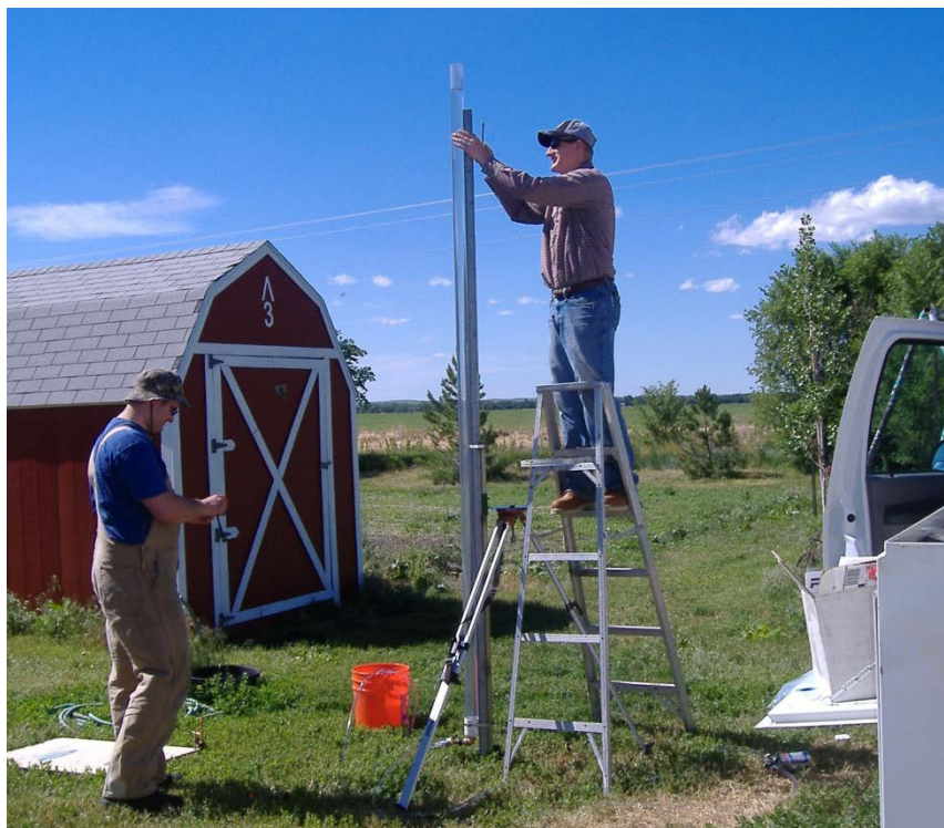
Figure 1. Calibration with water column
