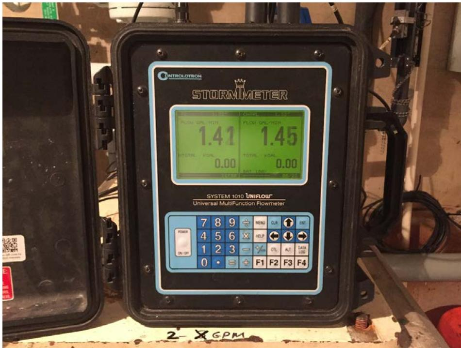
**Figure 6. Dual channel ultrasonic flow meter for monitoring bioboxes flowrates during testing**
