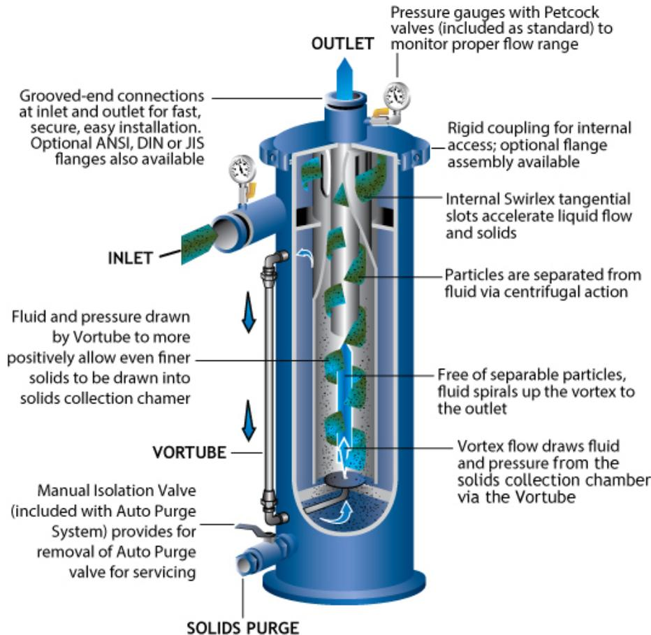
**Figure 1. Schematic of centrifugal separator (Lakos – Lindsey Corp)**
