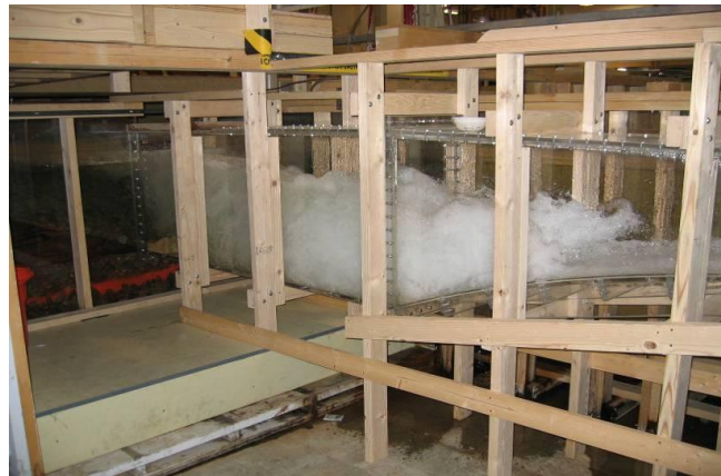
Figure 2. Choke Canyon stilling basin 1:10 scale model operating at 50% gate opening.
