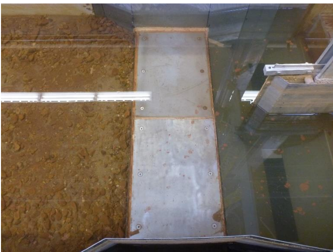
Figure 4. Instrumented impact plates installed in flume at USDA-ARS-NSL. Sediment sampling weigh pans are at the right of the photo with the 2-plate impact system in the center. Flow is from left to right.
