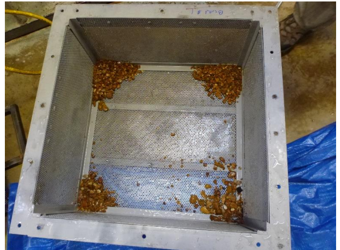
Figure 5. Gravel traps sampling particle size and mass. The sampling box shown is made from a metal screen material with 4 mm round holes.
